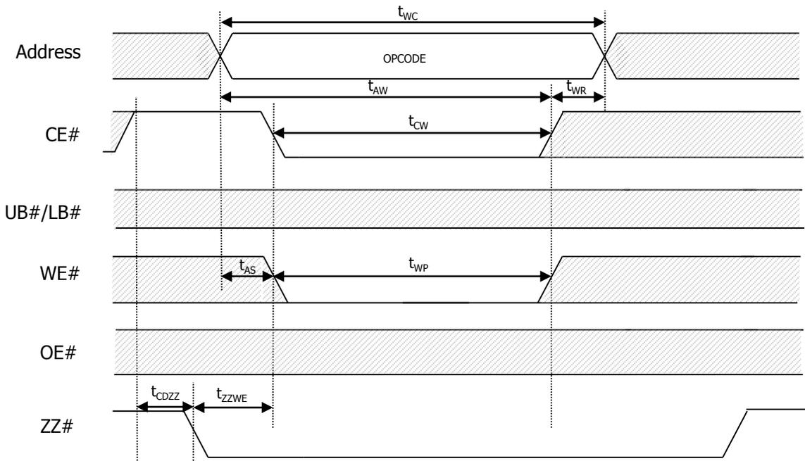
**Figure 12: DPD Entry and Exit Timing**
