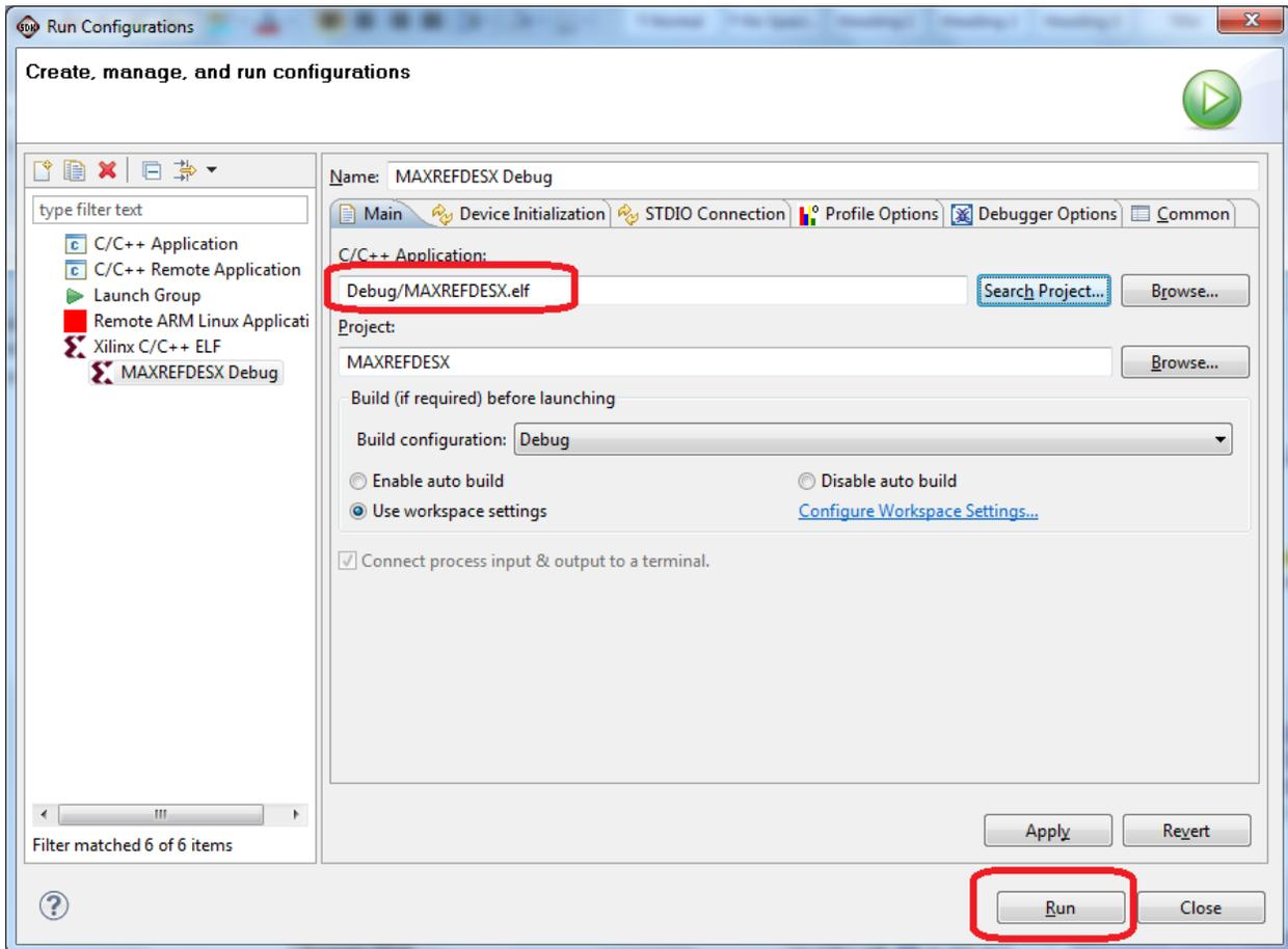
Once the Debug/MAXREFDES4 configuration is set up once, you just need to press the **Run** button if you ever want to run the program again.
