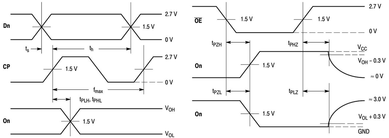
**WAVEFORM 1 - PROPAGATION DELAYS, SETUP AND HOLD TIMES**
