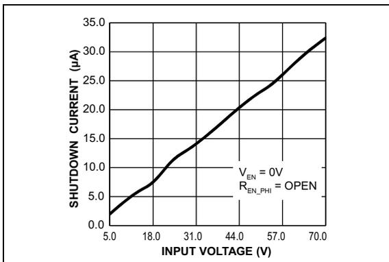
**FIGURE 2-2:**  $V_{IN}$  Shutdown Current vs. Input Voltage.
