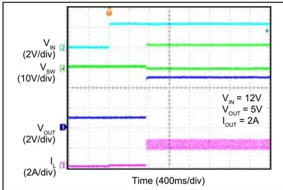
**FIGURE 2-31:**  $V_{IN}$  Start-Up with 1V Pre-Biased Output (MIC28512-2).
