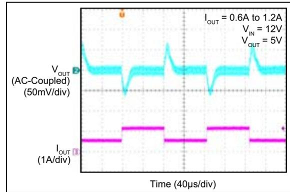
**FIGURE 2-58:** MIC28512-2 Load Transient Response (0.6A to 1.2A).
