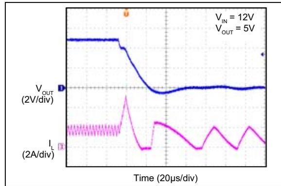
**FIGURE 2-36:** Short Circuit (MIC28512-2).
