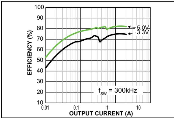
**FIGURE 2-13:** Efficiency ( $V_{IN} = 48V$ ) vs. Output Current (MIC28512-1).
