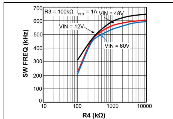
**FIGURE 5-3:** Switching Frequency vs. R4.
