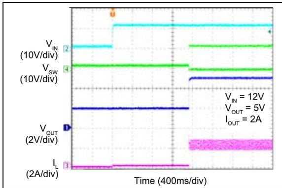
**FIGURE 2-32:**  $V_{IN}$  Start-Up with 2V Pre-Biased Output (MIC28512-2).
