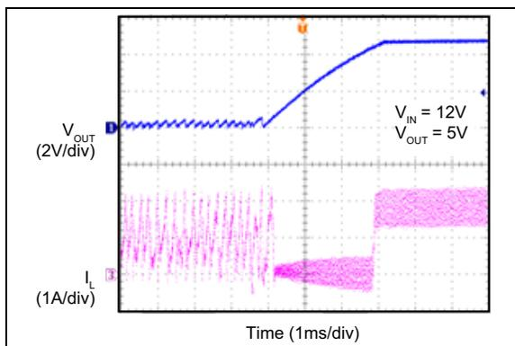
**FIGURE 2-39:** Output Recovery from Short Circuit to 2A.
