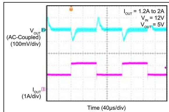
**FIGURE 2-60:** MIC28512-2 Load Transient Response (1.2A to 2A).
