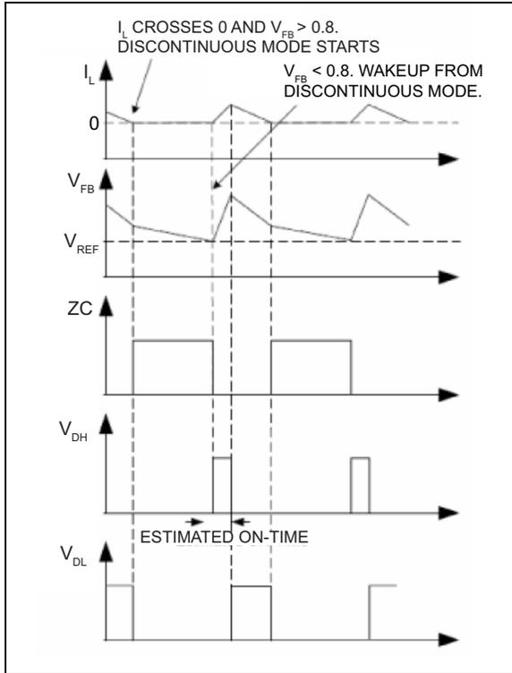
**FIGURE 4-4:** MIC28512-1 Control Loop Timing (Discontinuous Mode).
