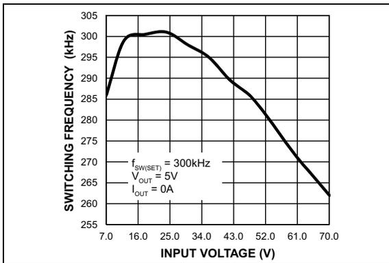
**FIGURE 2-26:** Switching Frequency vs. Input Voltage (MIC28512-2).
