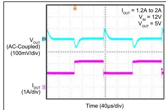
**FIGURE 2-59:** MIC28512-1 Load Transient Response (1.2A to 2A).
