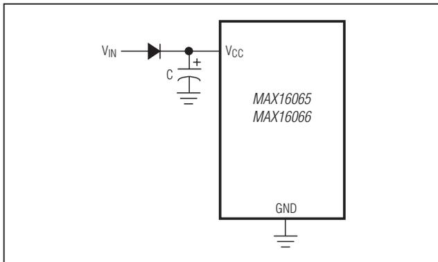
Figure 17. Power Circuit for Shutdown During Fault Conditions
