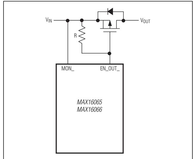
Figure 18. Connection for a p-Channel Series-Pass MOSFET
