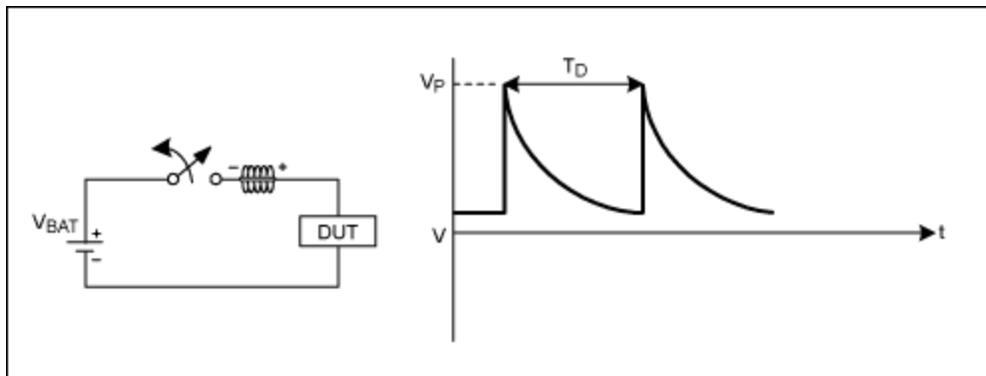
Figure 2. In response to repetitive switching action, this circuit produces positive repetitive pulses with amplitudes from +75V to +150V, and a typical duration of 50 $\mu$ s. A typical source impedance is 2 $\Omega$  to
