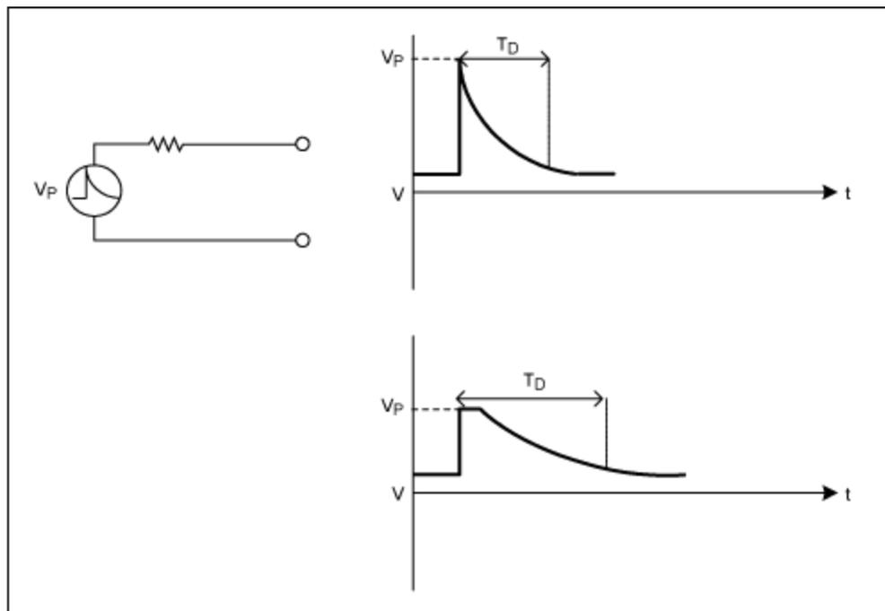
Figure 4. A load-dump pulse occurs when an alternator is suddenly disconnected while delivering high current to a discharged battery. The sudden reduction in current induces high voltage at the alternator output to maintain the energy in the system. The duration of this transient depends on the electrical time constant of the alternator field circuit and the regulator response time.
