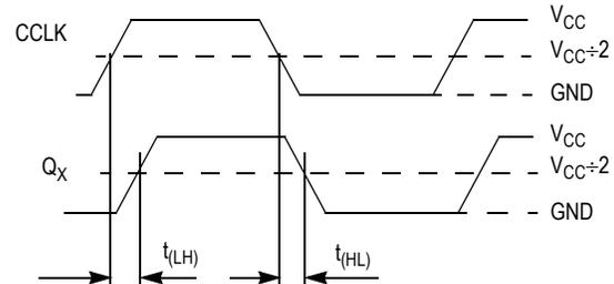
$$t_{SK(P)} = |t_{PLH} - t_{PHL}|$$
