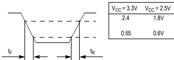
Figure 7. Output Transition Time Test Reference
