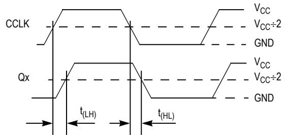
Figure 8. Propagation Delay ( $t_{PD}$ ) Test Reference
