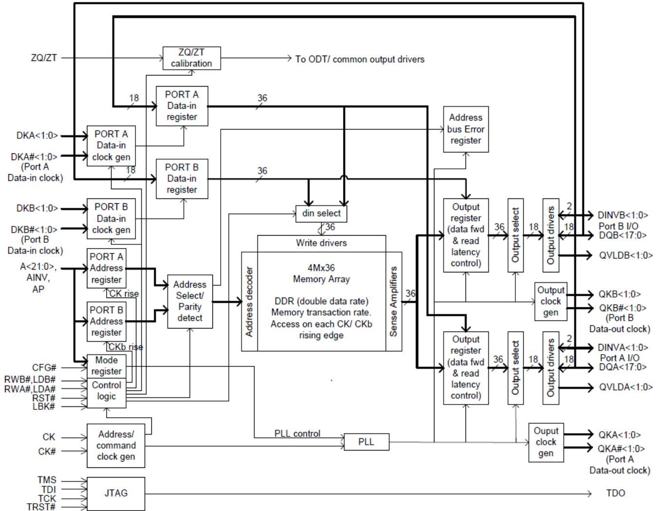
Logic Block Diagram – CY7C4141KV13
