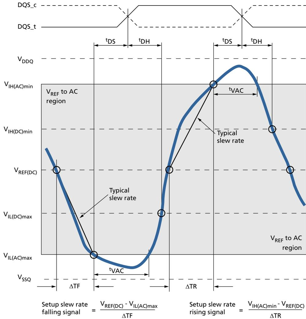
**Figure 71: Typical Slew Rate – t<sub>DH</sub> for DQ Relative to Strobe**
