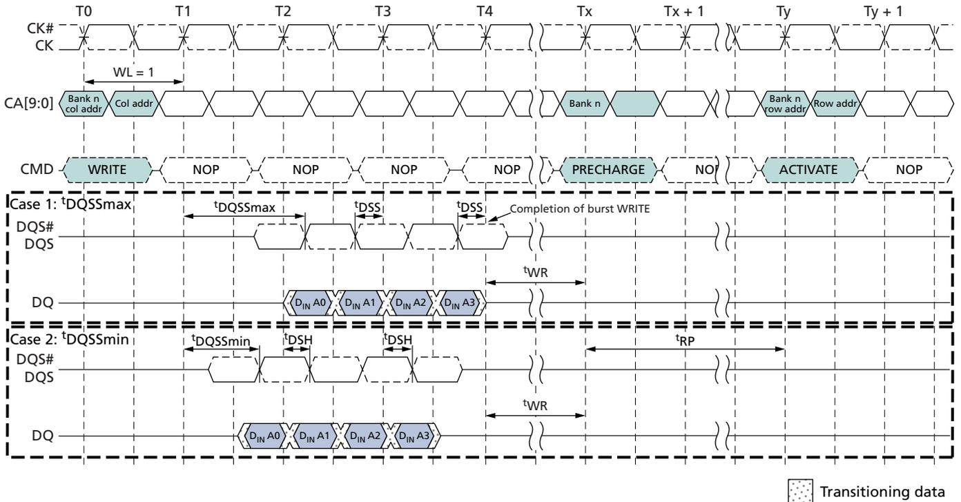
**Figure 25: Burst WRITE Followed by Burst READ – RL = 3, WL = 1, BL = 4**
