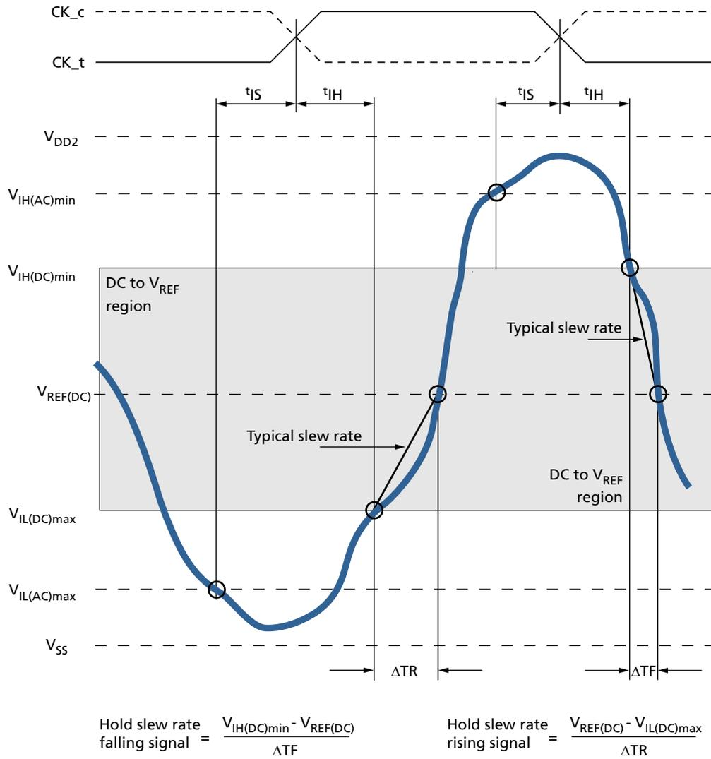
**Figure 68: Tangent Line -  $t_{IS}$  for CA and CS\_n Relative to Clock**
