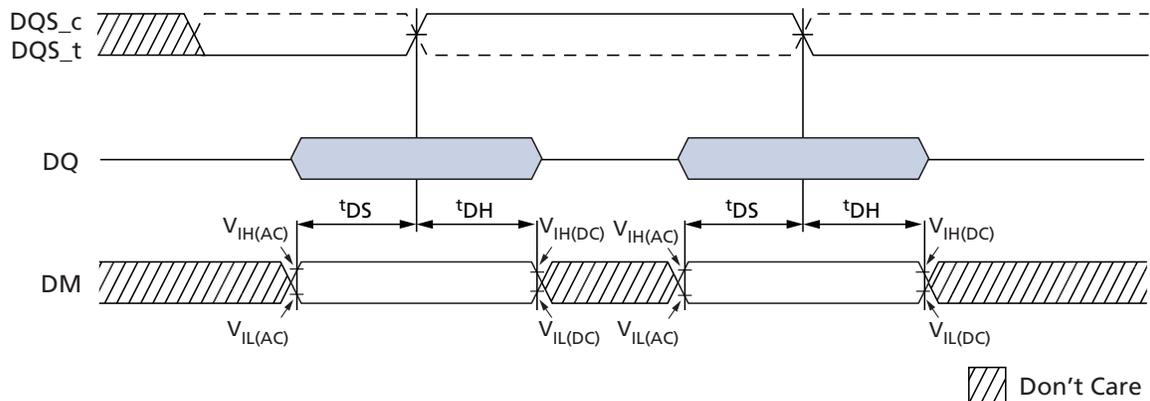
**Figure 31: Write Data Mask – Second Data Bit Masked**
