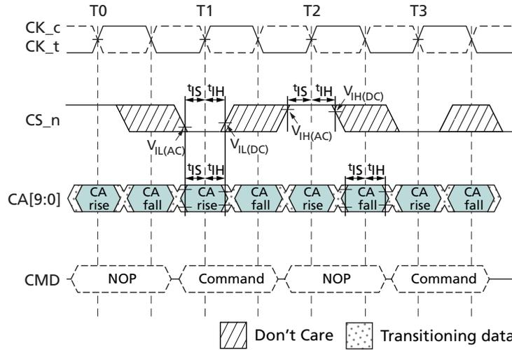
Note: 1. Setup and hold conditions also apply to the CKE pin. For timing diagrams related to the CKE pin, see the Power-Down section.
