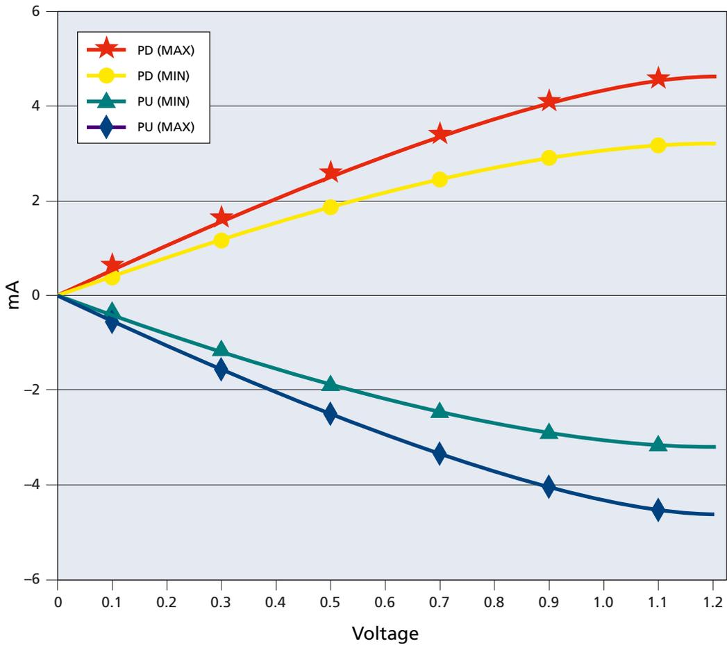
**Figure 65: Output Impedance = 240 Ohms, I-V Curves After Calibration**
