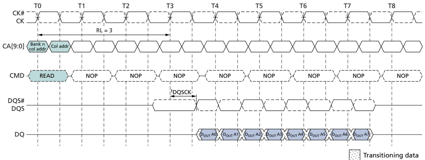
**Figure 17:  $t_{DQCKDL}$  Timing**
