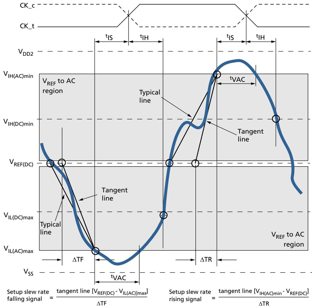
**Figure 69: Tangent Line – t<sub>IH</sub> for CA and CS\_n Relative to Clock**
