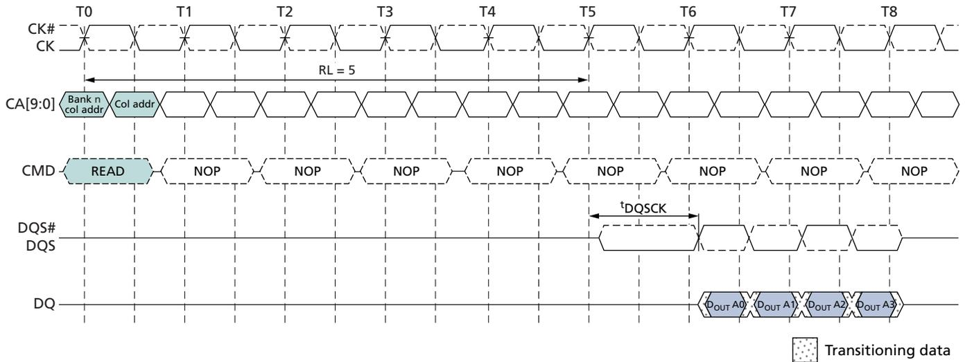
**Figure 16: Burst READ – RL = 3, BL = 8,  $t_{DQSCK} < t_{CK}$**
