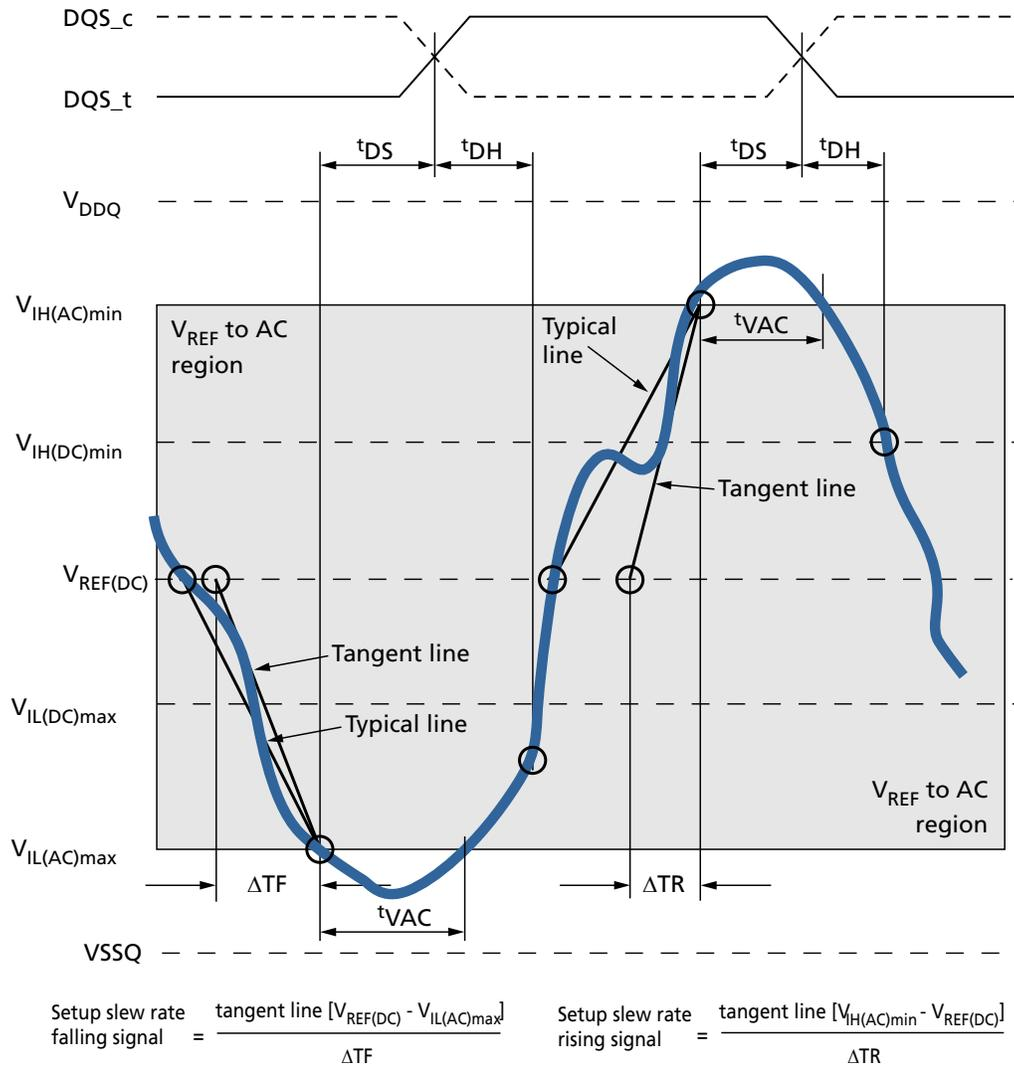
**Figure 73: Tangent Line – t<sub>DH</sub> for DQ with Respect to Strobe**
