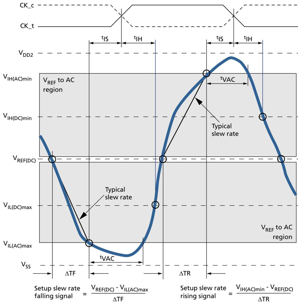
**Figure 67: Typical Slew Rate – t<sub>IH</sub> for CA and CS\_n Relative to Clock**
