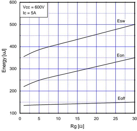
**Fig 9. Typical Switching Loss vs. Gate Resistance**
