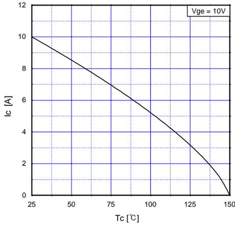
**Fig 3. Maximum Collector Current vs. Case Temperature**
