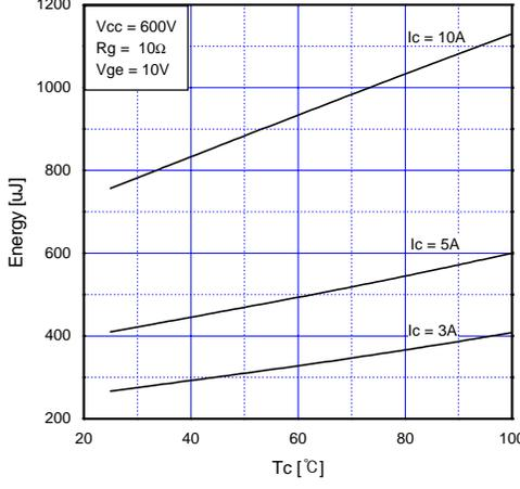
**Fig 10. Typical Switching Loss vs. Case Temperature**
