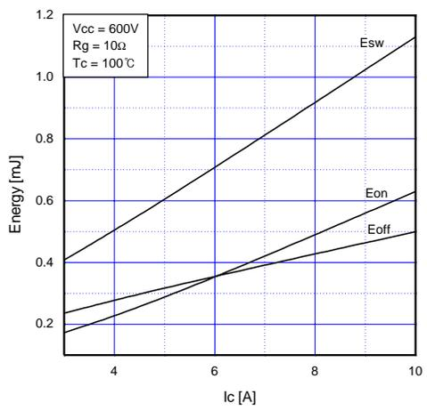
**Fig 11. Typical Switching Loss vs. Collector Current**
