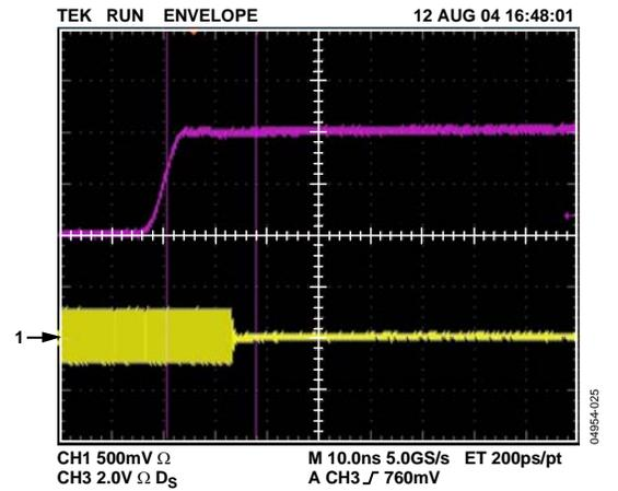
Figure 25. Power Shutdown Response Time, RF = 380 MHz
