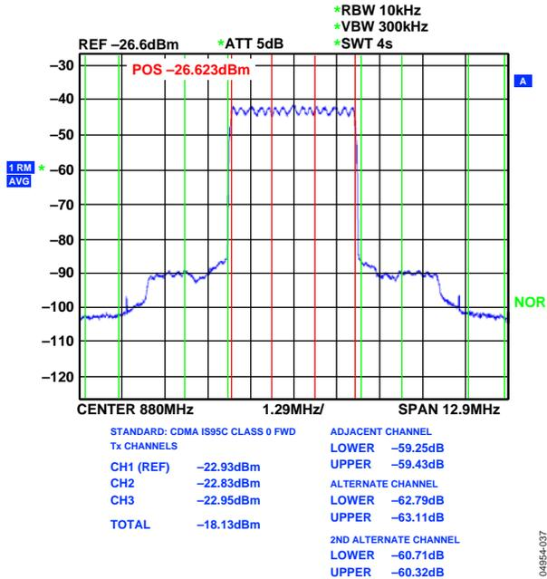
Figure 41. ADL5390 as a Quadrature Modulator with the Use of an External 90°Phase Splitter, RF/LO Power = -1 dBm and Gain Control Inputs Driven Differentially with 0.353 V<sub>p,p</sub>, 3-Carrier CDMA2000 I/Q Data
