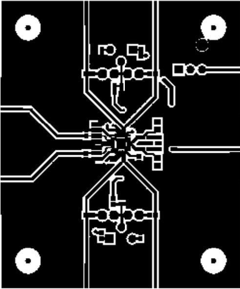
Figure 45. Component Side Layout
