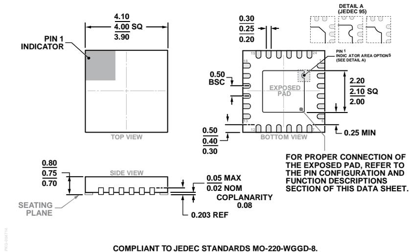
Figure 47. 24-Lead Lead Frame Chip Scale Package [LFCSPP]
