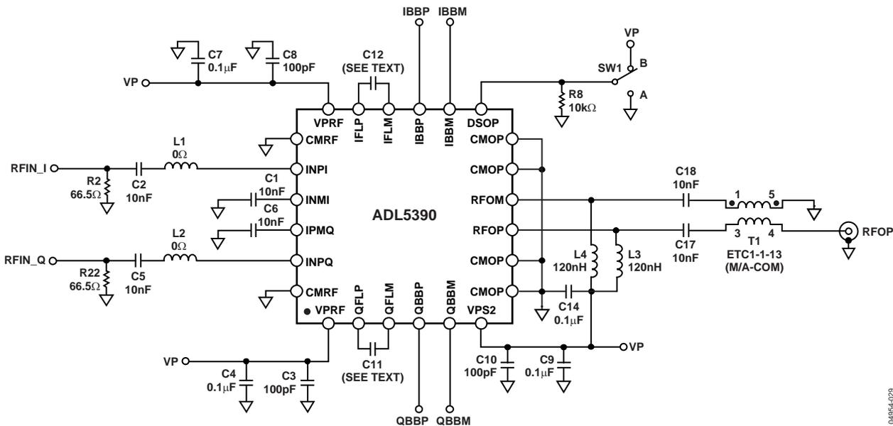
Figure 29. Basic Connections
