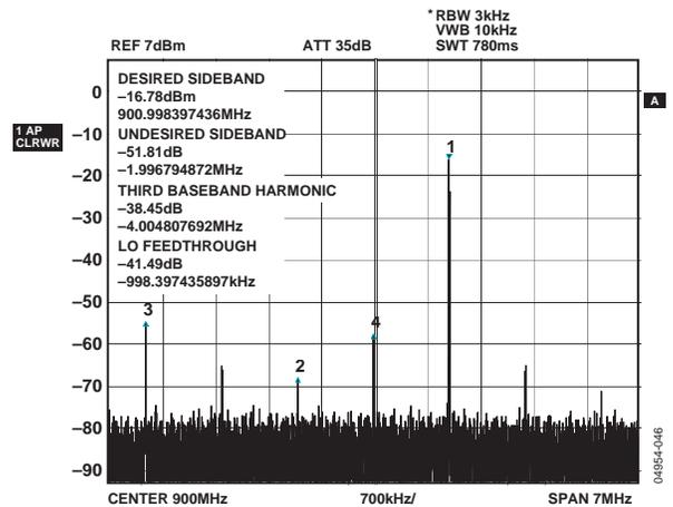
Figure 40. SSB Modulator Applications with Gain and Phase Errors Corrected,  $RF P_{in} = -15 \text{ dBm}$ ,  $V_{IBB} = V_{QBB} = 0.5 \text{ V}$  (With Reference to a Common-Mode Voltage of 0.5 V), I/Q Phase Offset by 3°, and Magnitude Offset by 0.5 V
