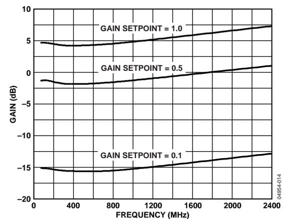
Figure 14. Gain vs. RF Frequency, Gain Setpoint = 1.0, 0.5, 0.1
