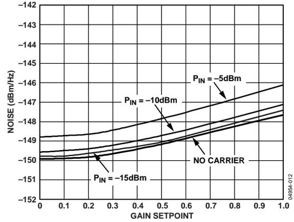
Figure 12. Output Noise Floor vs. Gain Setpoint, No Carrier, with Carrier (20 MHz Offset), RF P<sub>IN</sub> = -5, -10, -15, No Carrier, RF Frequency = 380 MHz
