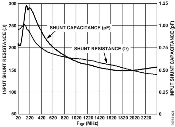
Figure 21. S11 of RF Input (Shunt R/C Representation)
