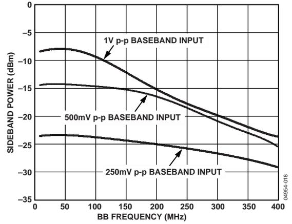
Figure 18. IQ Modulation Bandwidth vs. Baseband Magnitude
