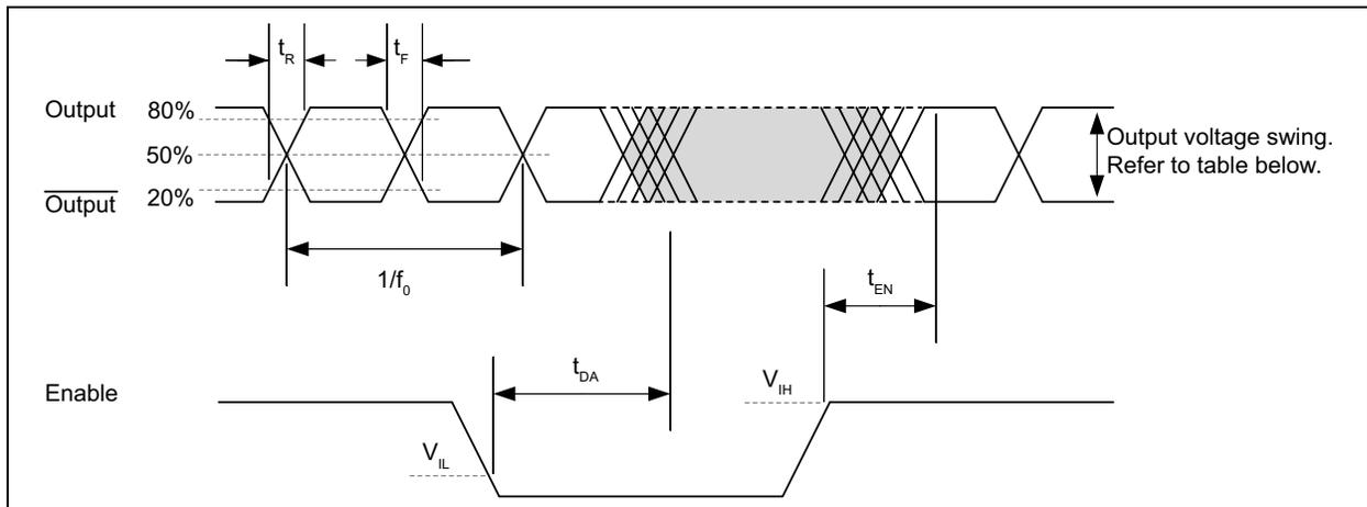
**FIGURE 4-1:** LVPECL, LVDS, and HCSL Output Waveform.
