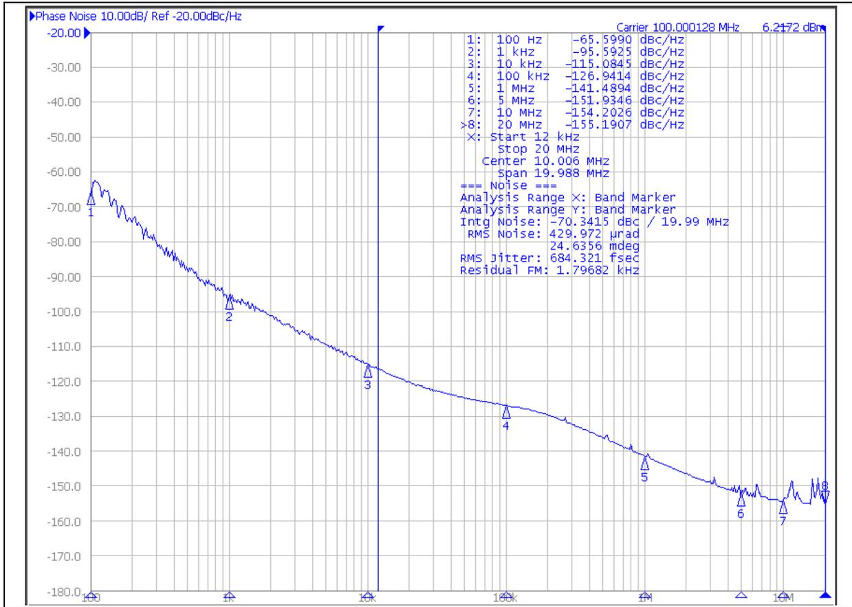
FIGURE 8-1: DSC12x4 Phase Noise at 100 MHz.
