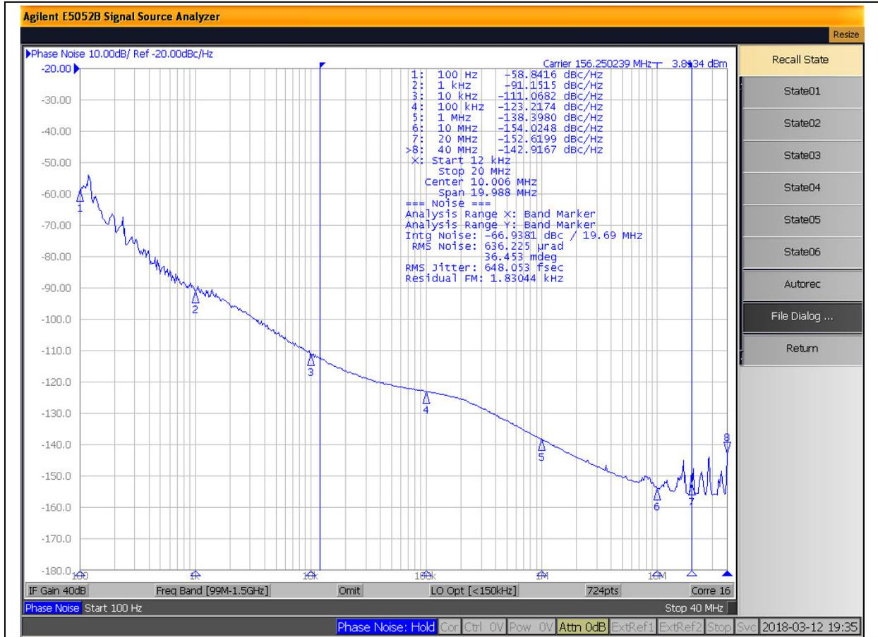
**FIGURE 8-2:** DSC12x2 Phase Noise at 156.25 MHz.
