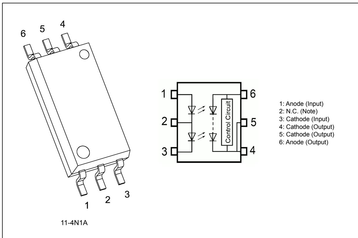
Note: Input side is considered 2 LEDs serial connection.(i.e. Forward mean pin 1 to 3, Reverse mean pin 3 to 1.) Don't connect anything to pin 2.
