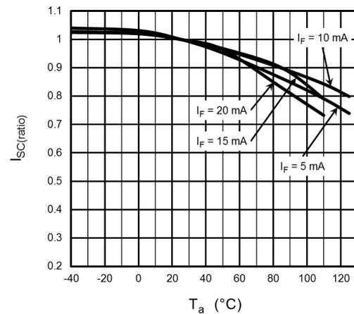
Fig. 12.10  $I_{SC}(\text{ratio}) - T_a$
