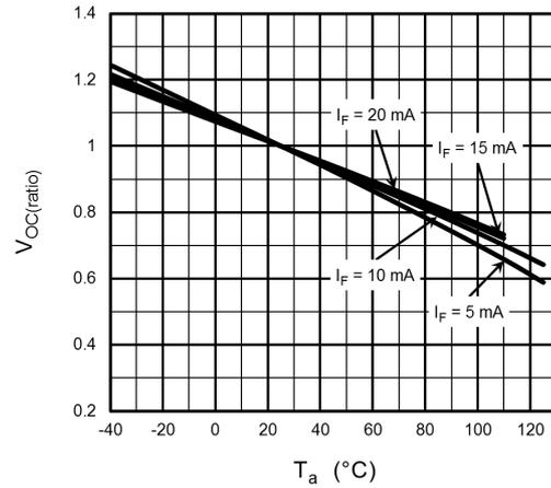
Fig. 12.8  $V_{OC}(\text{ratio}) - T_a$
