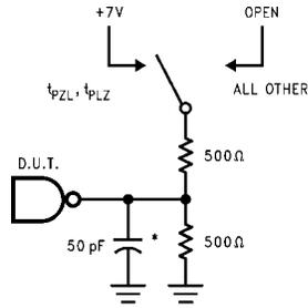
\*Includes jig and probe capacitance
