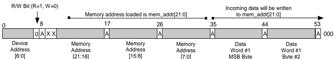
Figure 10 Write protocol with 7-bit Slave Address (ADS=0). I<sup>2</sup>C writes to memory align on 32-bit word boundaries, thus the 22 address MSBs must be provided while the 2 LSB's associated with word and byte pointers are DON'T CARE and are therefore not transmitted.
