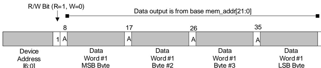
Figure 11 Read protocol with 7-bit Slave Address (ADS=0)
