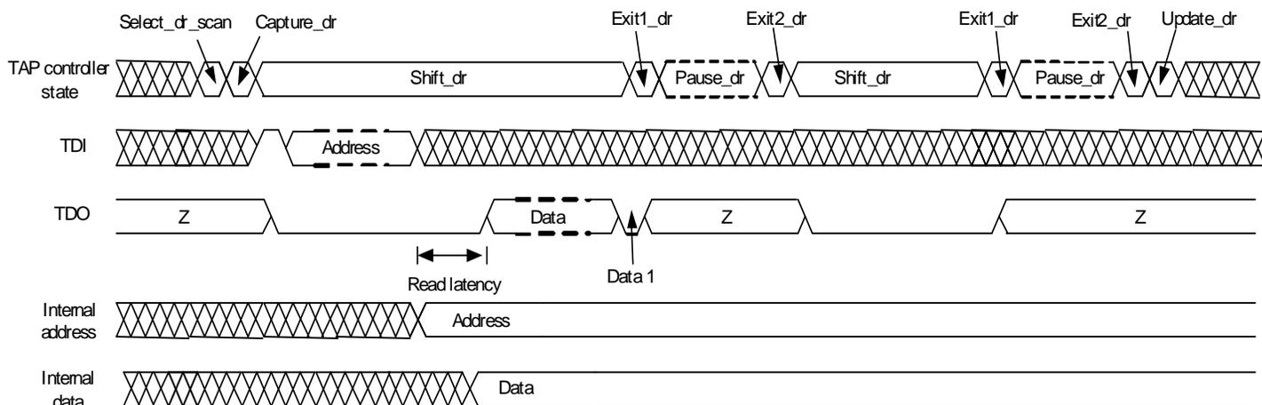
Figure 26 Implementation of read during configuration register access
