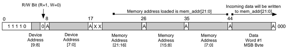
Figure 8 Write protocol with 10-bit Slave Address (ADS =1). I<sup>2</sup>C writes to memory align on 32-bit word boundaries, thus the 22 address MSBs must be provided while the 2 LSB's associated with word and byte pointers are DON'T CARE and are therefore not transmitted.
