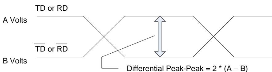
Figure 14 Differential Peak-Peak Voltage of Transmitter or Receiver
