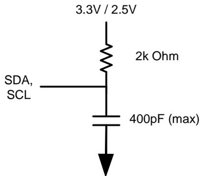
Figure 6 AC Output Test Load (I<sup>2</sup>C)
