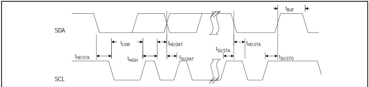
Figure 12 I<sup>2</sup>C Timing Waveforms14 Interrupt ( $\overline{\text{IRQ}}$ ) Electrical Specifications
