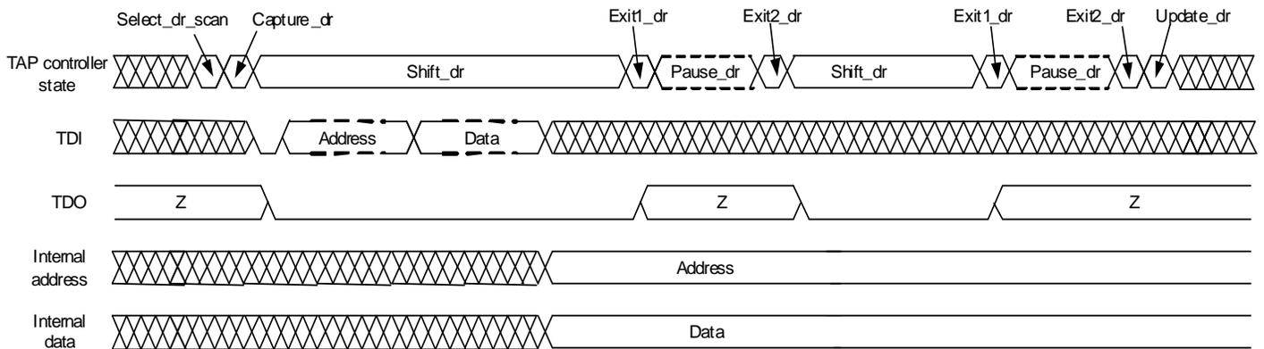
Figure 25 Implementation of write during configuration register access
