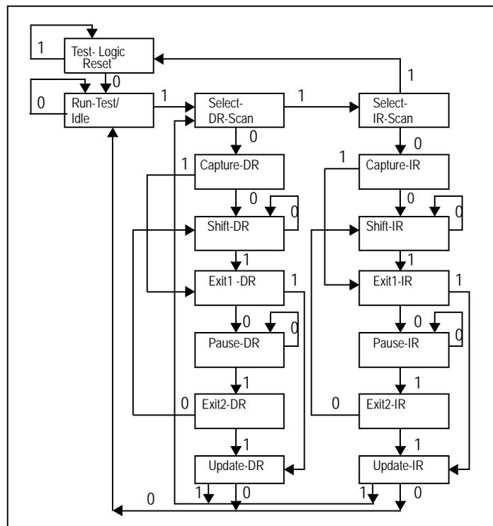
Figure 20 State Diagram of the CPS-16's TAP Controller
