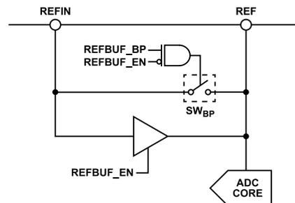
**Figure 74. Internal Reference Buffer Simplified Schematic**
