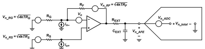
Figure 113. Noise Sources in Typical ADC AFE Circuit
