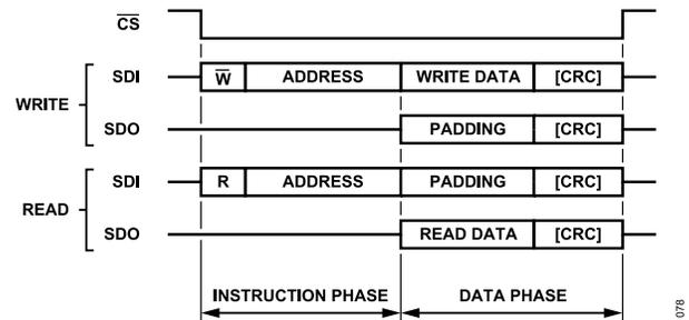
Figure 81. Basic SPI Frame
