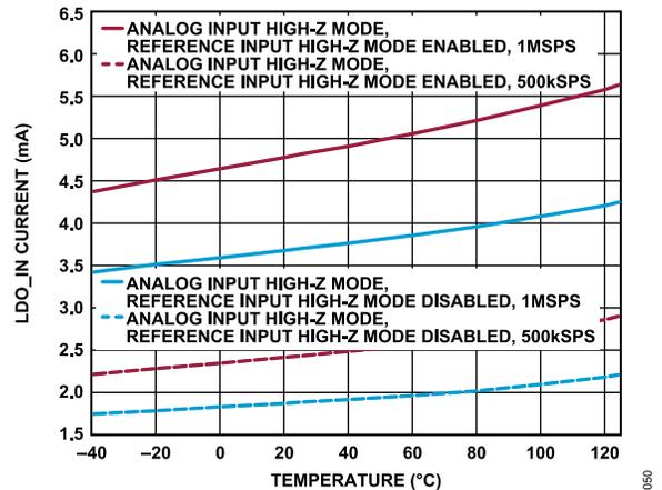
Figure 51. LDO\_IN Current vs. Temperature, Internal LDO Enabled
