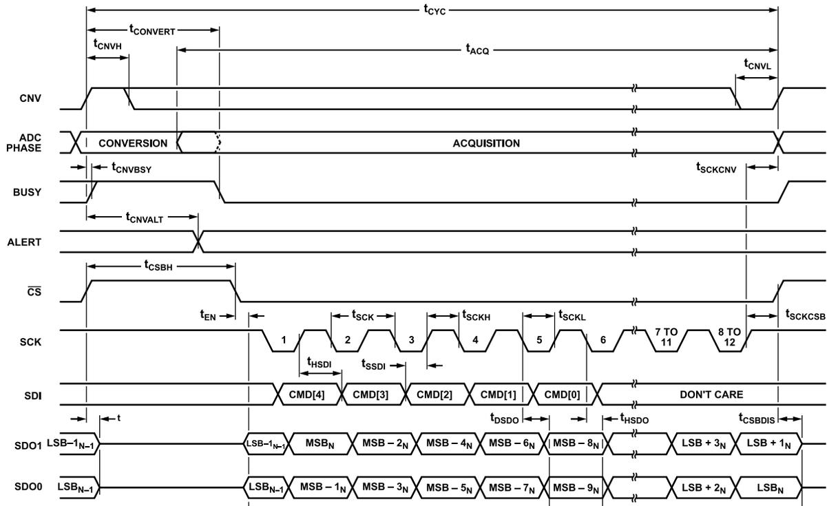
Figure 96. Conversion Mode Timing Diagram, Dual-SDO Mode, SDO\_STATE = 0
