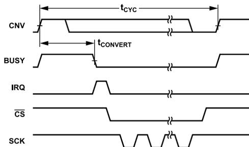
Figure 123. SPI Synchronization with Busy Indicator
