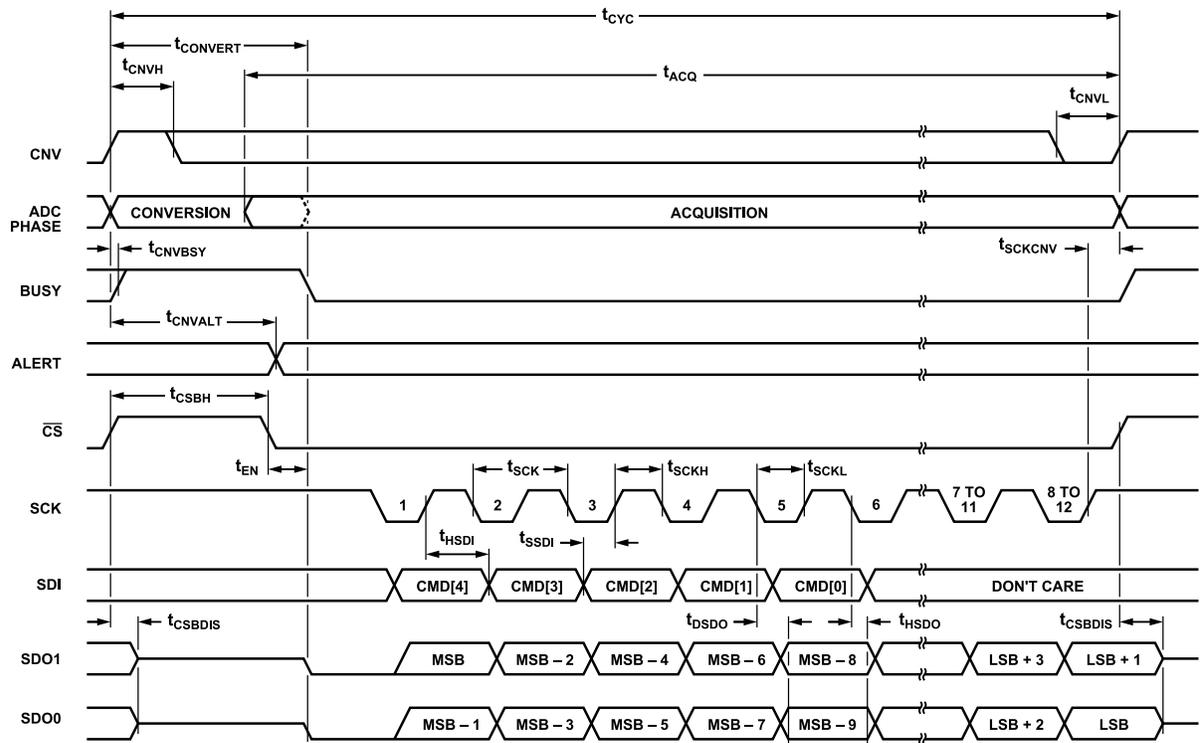
Figure 97. Conversion Mode Timing Diagram, Dual-SDO Mode, SDO\_STATE = 1
