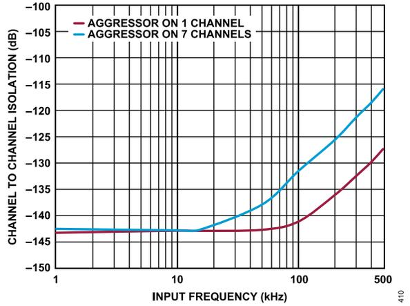
Figure 37. Channel to Channel Isolation vs. Input Frequency
