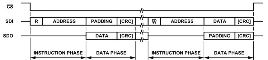
Figure 89. Single Instruction Mode SPI Frame
