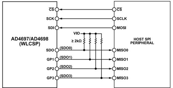
Figure 120. AD4697/AD4698 SPI Connection Diagram (Quad-SDO Mode)
