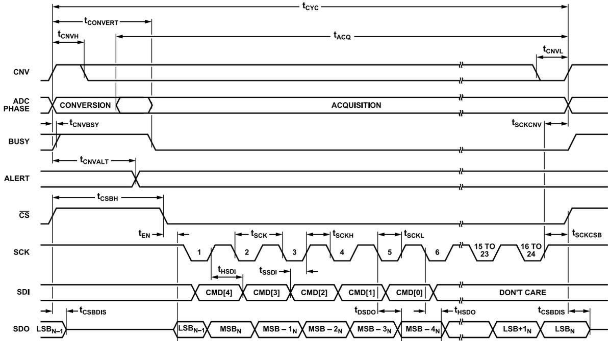
Figure 94. Conversion Mode Timing Diagram, Single-SDO Mode, SDO\_STATE = 0
