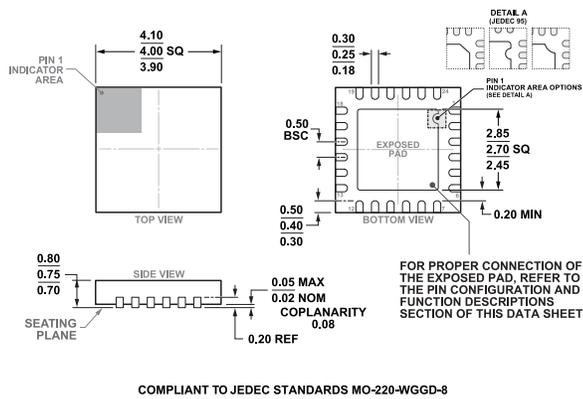
**Figure 128. 24-Lead Lead Frame Chip Scale Package [LFCSP]
