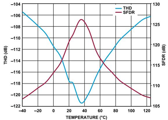
Figure 26. THD and SFDR vs. Temperature,  $f_{IN} = 1$  kHz
