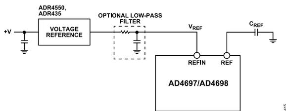
Figure 117. Typical Connection Diagram for Driving REFIN Input
