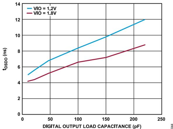
Figure 60.  $t_{DSO}$  vs. Digital Output Load Capacitance
