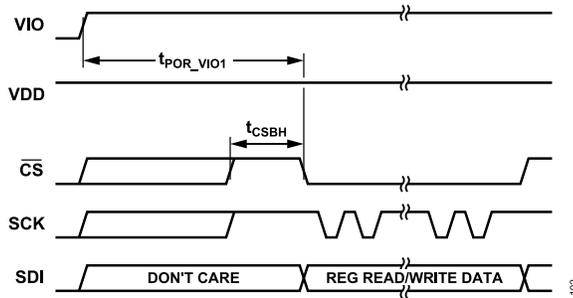
Figure 107. VIO POR Timing Diagram (VDD Supplied Externally)
