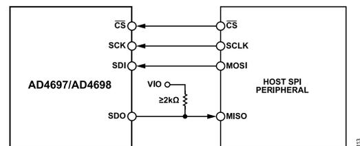
Figure 118. AD4697/AD4698 SPI Connection Diagram (Single-SDO Mode)
