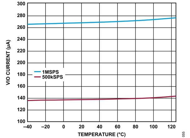
Figure 56. VIO Current vs. Temperature, Conversion Mode, OSR = 1
