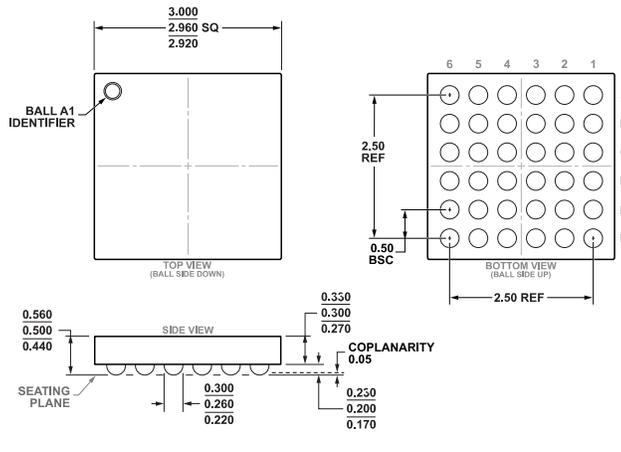
**Figure 129. 36-Ball Wafer Level Chip Scale Package [WLCSP]
