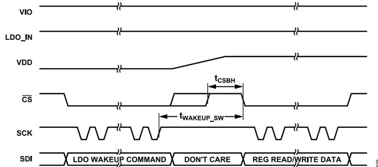
Figure 110. LDO Wake-Up Command POR Timing Diagram
