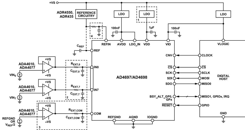
1. DEDICATED +1.8V SUPPLY FOR VDD NOT REQUIRED WHEN USING INTERNAL LDO
