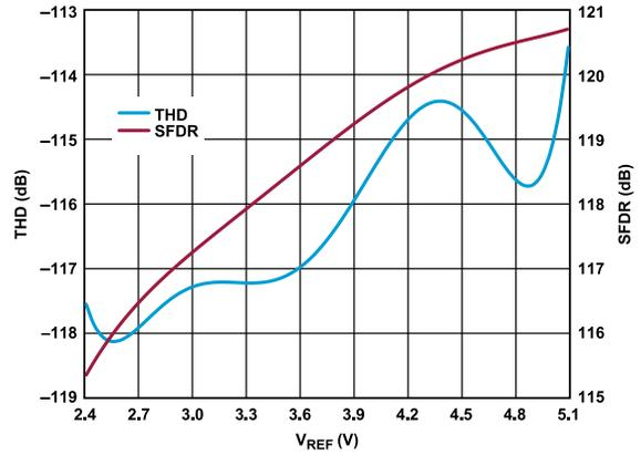
Figure 25. THD and SFDR vs.  $V_{REF}$ ,  $f_{IN} = 1$  kHz
