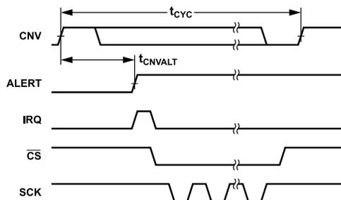
Figure 124. SPI Synchronization with Alert Indicator
