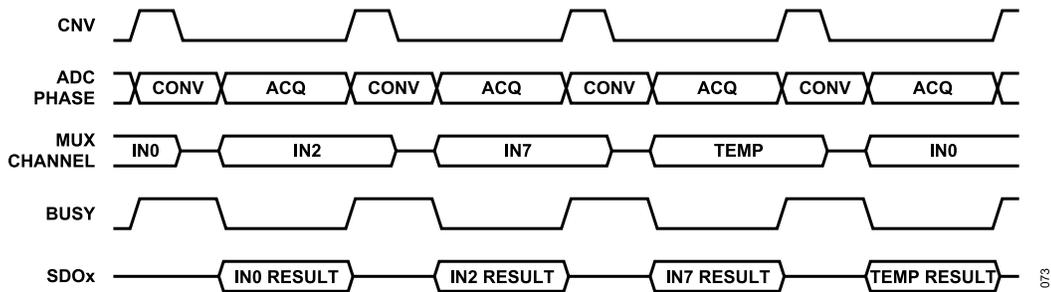
Figure 76. Standard Sequencer Example with OSR = 1
