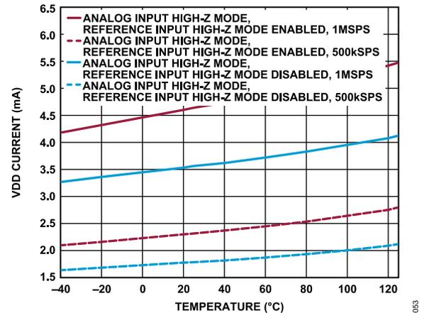
Figure 54. VDD Current vs. Temperature, Internal LDO Disabled
