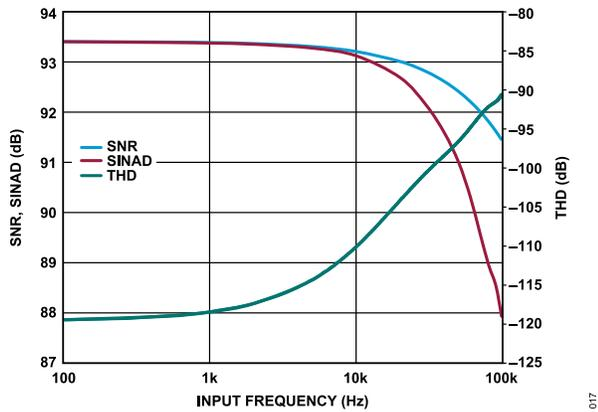
Figure 18. SNR, SINAD, and THD vs. Input Frequency
