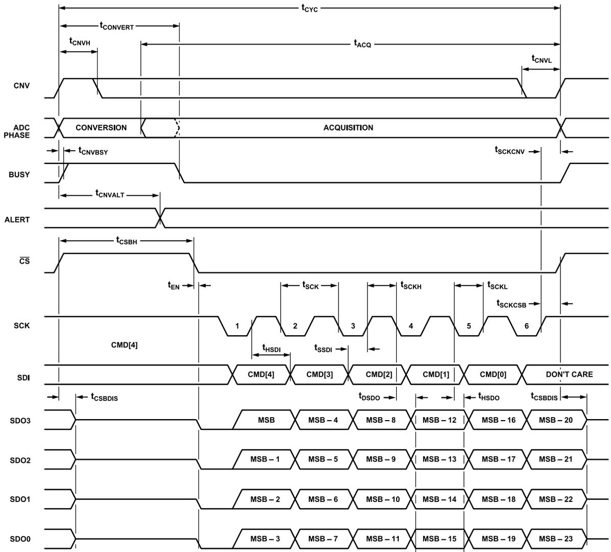
Figure 99. Conversion Mode Timing Diagram, Quad-SDO Mode, SDO\_STATE = 1
