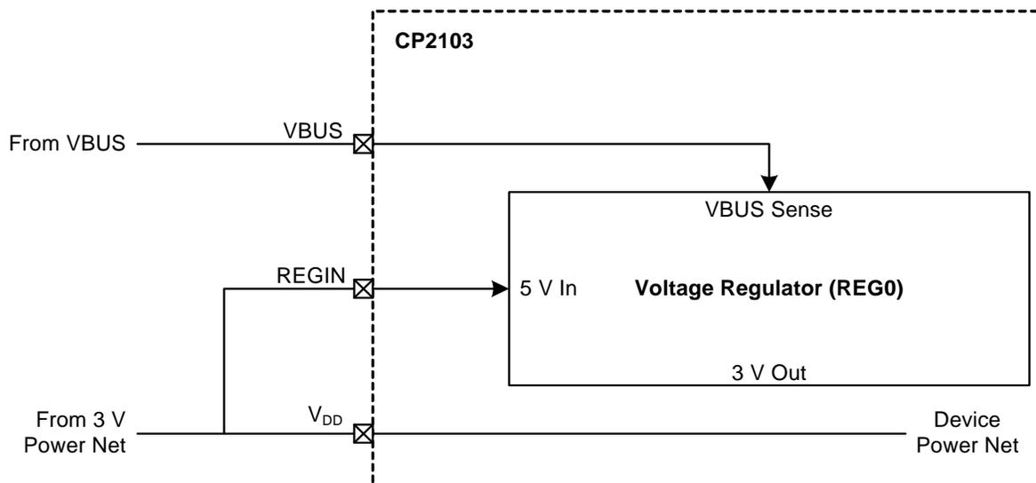
Figure 9. Configuration 3: USB Self-Powered, Regulator Bypassed
