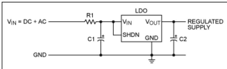
Figure 3a. Single RC ripple filter.
