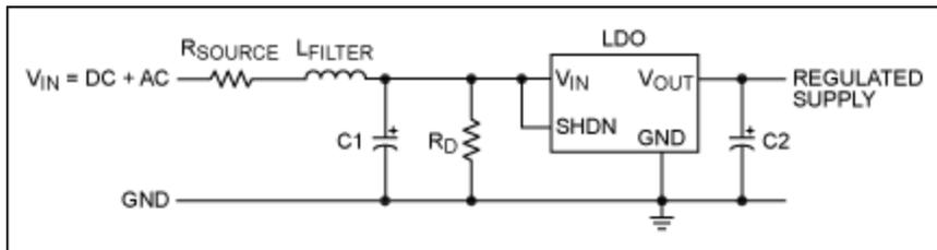
Figure 4b. Illustrating the position of damping resistor.
