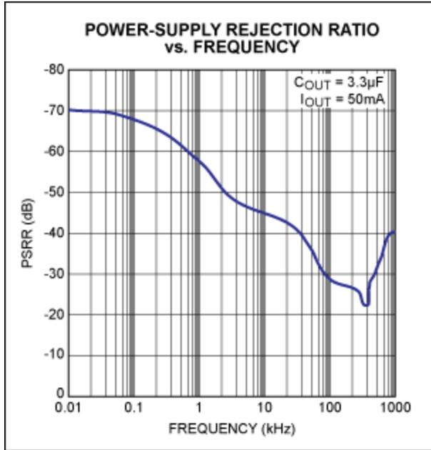
Figure 2. MAX1792 PSRR characteristic.
