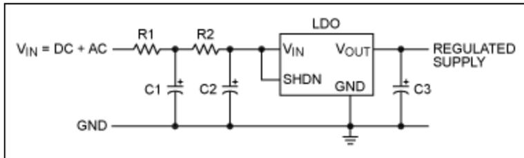
Figure 3b. Second-order cascade RC ripple filter.
