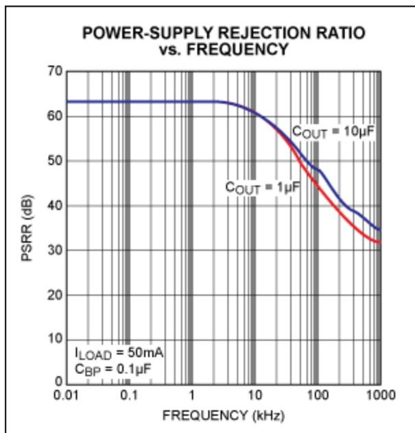
Figure 1. MAX8867 PSRR characteristic.
