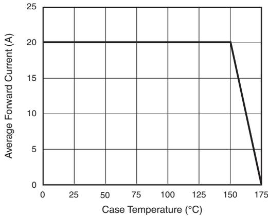
Fig. 1 - Forward Current Derating Curve (Total)
