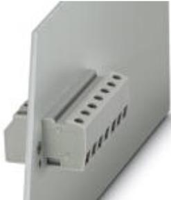
Panel feed-through terminal block, Connection method: Screw connection, Screw connection, Load current : 41 A, Cross section: 0.2 mm<sup>2</sup> - 6 mm<sup>2</sup>, AWG 24 - 10, Connection direction of the conductor to plug-in direction: 0 °, Width: 8.1 mm, Color: gray
