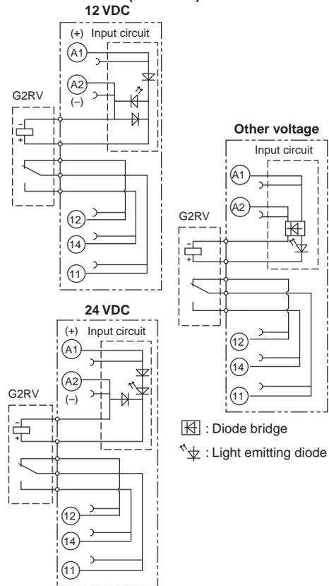
**Models with latching lever (with test switch)**
