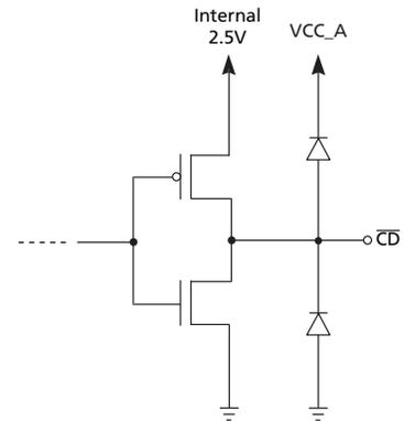
Figure 3-6:  $\overline{CD}$  Circuit
