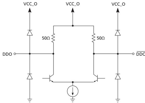
Figure 3-3: Output Circuit
