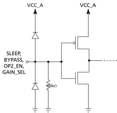
Figure 3-4: SLEEP, BYPASS, OP2\_EN and GAIN\_SEL Circuits
