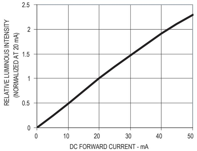
Figure 3. Relative luminous intensity vs. forward current
