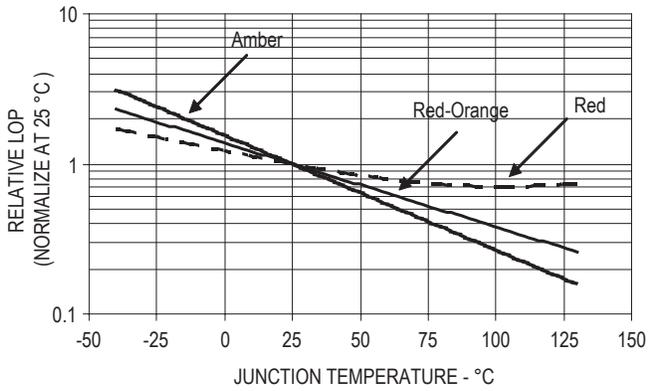
**Figure 8. Relative light output vs. junction temperature**
