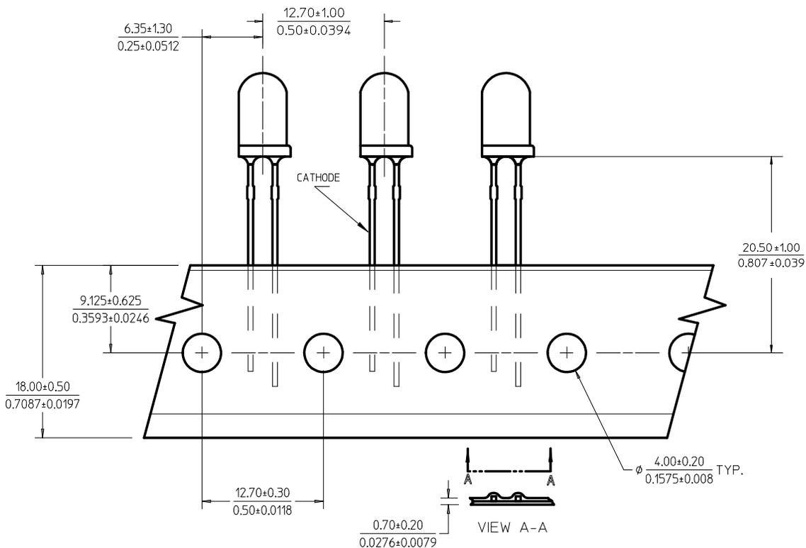
Note: The ammo-packs drawing is applicable for packaging option -DD & -ZZ and regardless standoff or non-standoff
