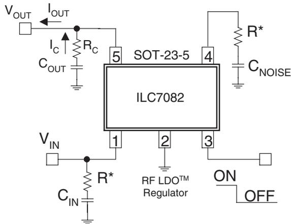
Figure 5. ESR Present in  $C_{OUT}$  and  $C_{NOISE}$
