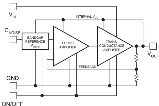
Figure 2. ILC7082 RF LDO Regulator Block Diagram
