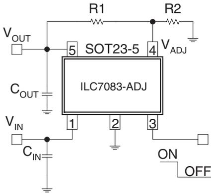
**Figure 3. Application Circuit for Adjustable Output Voltage**
