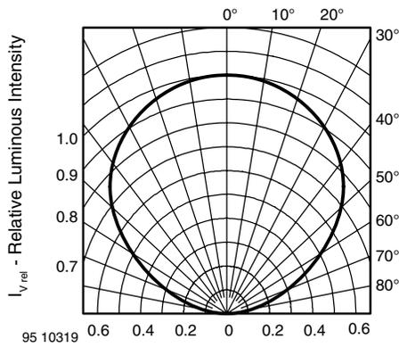
Figure 3. Rel. Luminous Intensity vs. Angular Displacement
