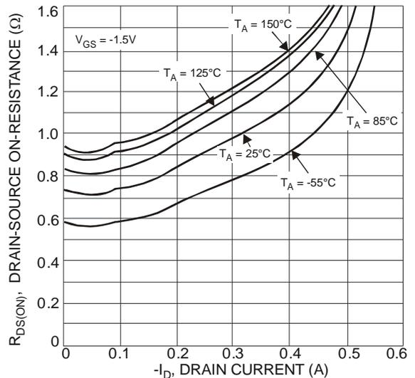
Fig. 9 Typical On-Resistance vs. Drain Current and Temperature
