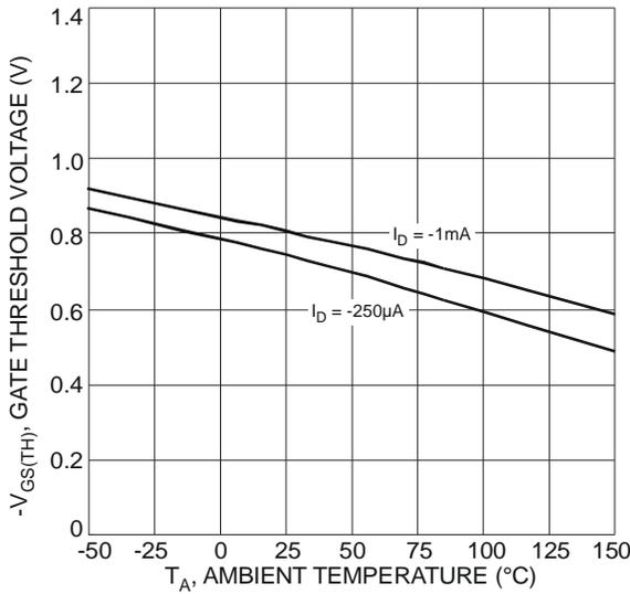
Fig. 12 Gate Threshold Variation vs. Ambient Temperature
