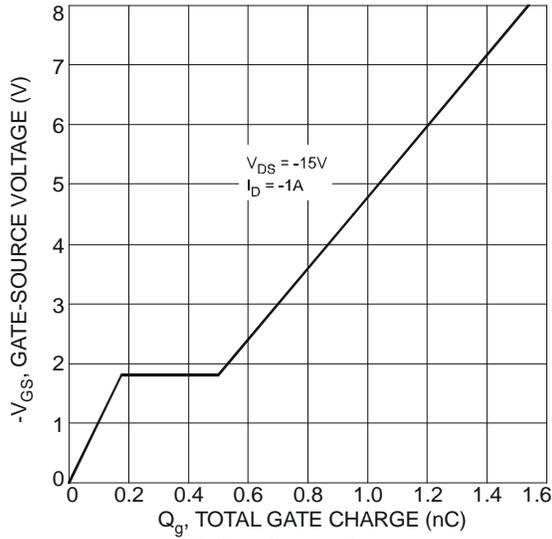
Fig. 18 Gate-Charge Characteristics
