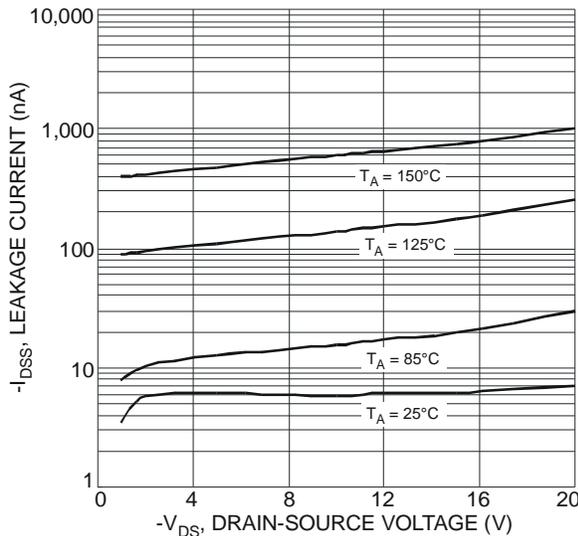
Fig. 14 Typical Leakage Current vs. Drain-Source Voltage
