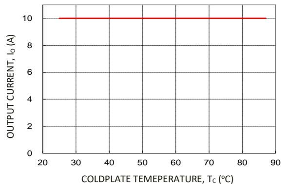
**Figure 22. Derated Output Current versus Cold Wall Temperature with local ambient temperature around module at 85C; V<sub>IN</sub>=24V or 48V.**
