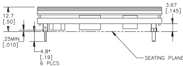
\*For optional pin lengths, see Table 2, Device Coding Scheme and Options
