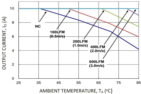
**Figure 18. Output Current Derating for the Open Frame Module; Airflow in the Transverse Direction from V<sub>out</sub>(-) to V<sub>out</sub>(+); V<sub>IN</sub>=24V, V<sub>O</sub>=12V.**
