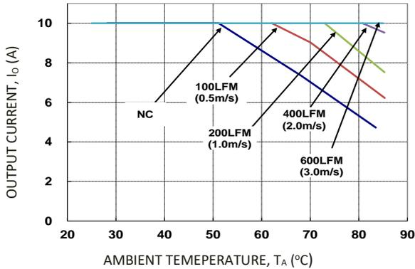
**Figure 17. Output Current Derating for the Module with 18H Heatplate; Airflow in the Transverse Direction from V<sub>out</sub>(-) to V<sub>out</sub>(+); V<sub>IN</sub>=48V, V<sub>O</sub>=12V**
