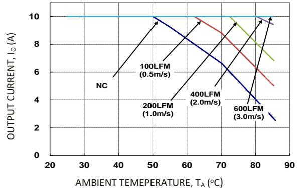
**Figure 20. Output Current Derating for the Module with 18 Heatplate; Airflow in the Transverse Direction from V<sub>out</sub>(-) to V<sub>out</sub>(+); V<sub>IN</sub>=24V, V<sub>O</sub>=12V.**
