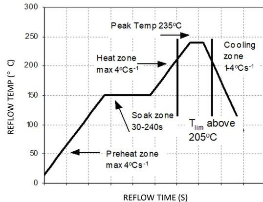
Figure 24. Reflow Profile for Tin/Lead (Sn/Pb) process.
