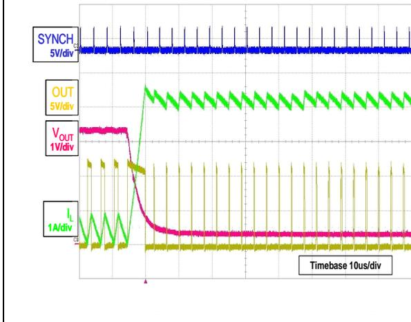
Figure 33. Short-circuit behavior  $V_{IN} = 24\text{ V}$
