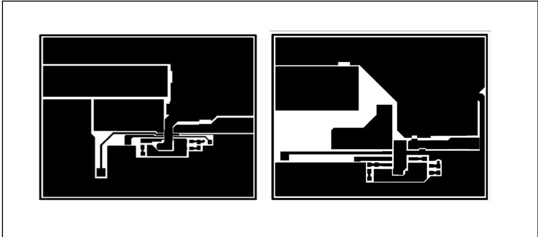
Figure 20. PCB layout: L7986 and L7986A (bottom side)
