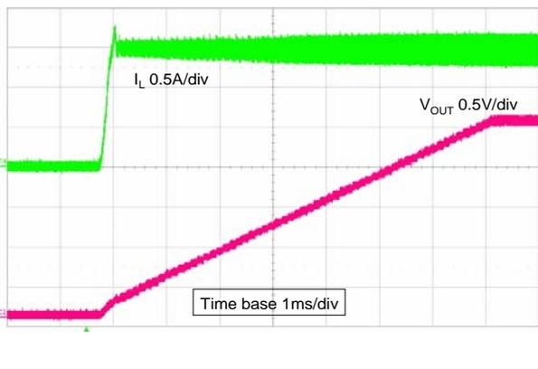
Figure 32. Short-circuit behavior  $V_{IN} = 12\text{ V}$
