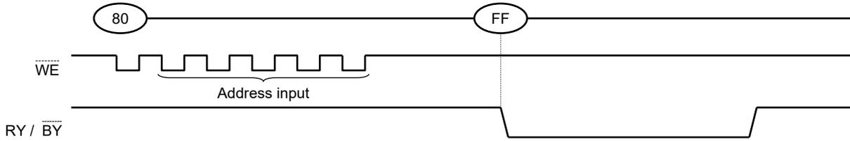
If a command other than “85h”, “10h”, “11h”, “15h” or “FFh” is input, the Program operation is not performed and the device operation is set to the mode that the input command specifies.
