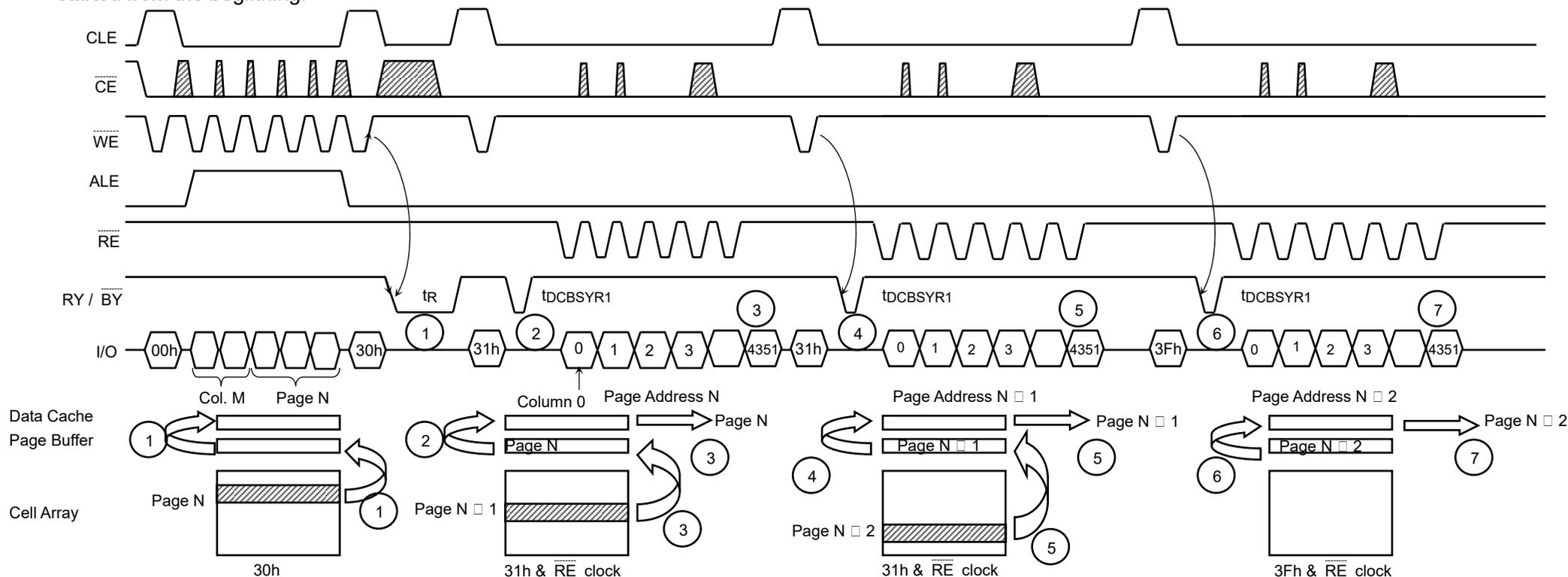
If the 31h command is issued to the device, the data content of the next page is transferred to the Page Buffer during serial data out from the Data Cache, reducing the  $t_R$  (Data transfer from memory cell to data register).
