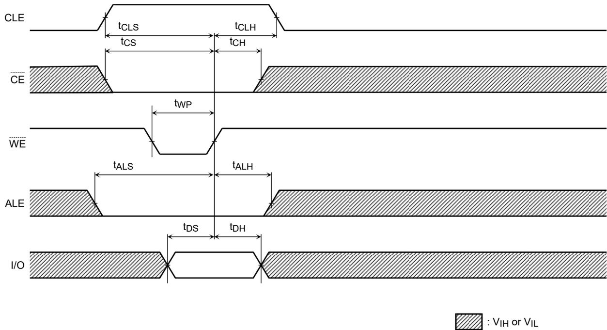
Address Input Cycle Timing Diagram
