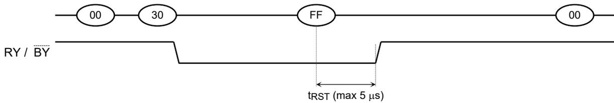
When a Reset (FFh) command is input during Ready
