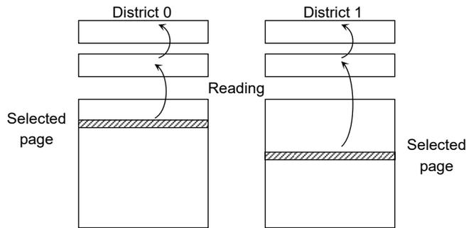
The data transfer operation from the cell array to the Data Cache via Page Buffer starts on the rising edge of WE in the 30h command input cycle (after the 2 Districts' address information has been latched). The device will be in the Busy state during this transfer period. After the transfer period, the device returns to Ready state. Serial data can be output synchronously with the  $\overline{RE}$  clock from the start address designated in the address input cycle.
