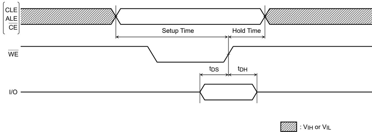
Command Input Cycle Timing Diagram
