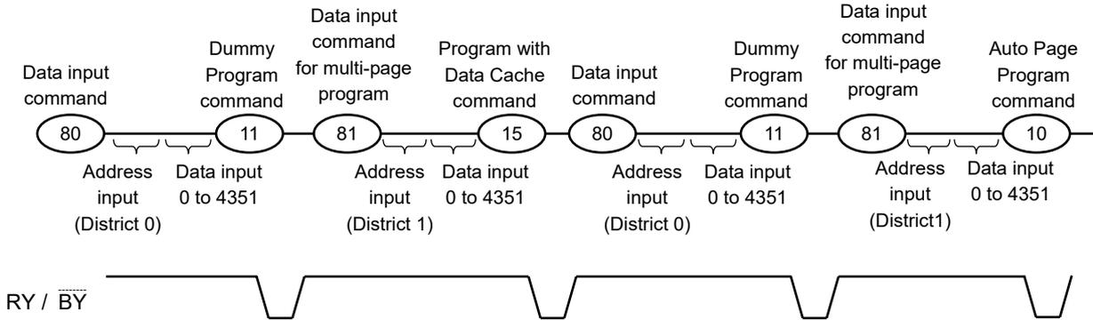
After either “15h” or “10h” Program command is input to the device, physical programming starts as follows. For details about Auto Page Program with Data Cache, refer to “Auto Page Program Operation with Data Cache”.
