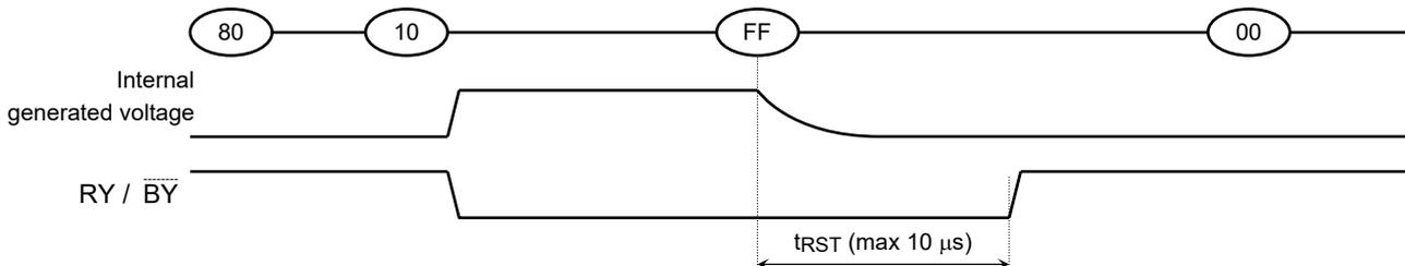
When a Reset (FFh) command is input during Erase operation
