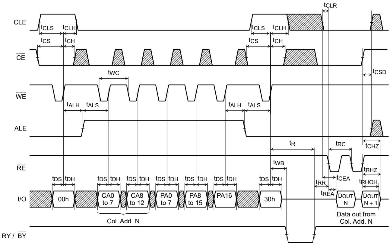
Read Cycle with Data Cache Timing Diagram (1/2)
