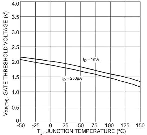
Fig. 8 Gate Threshold Variation vs. Junction Temperature
