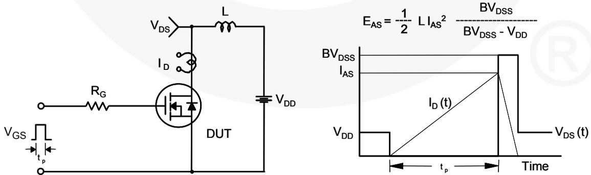
Figure 14. Unclamped Inductive Switching Test Circuit & Waveforms
