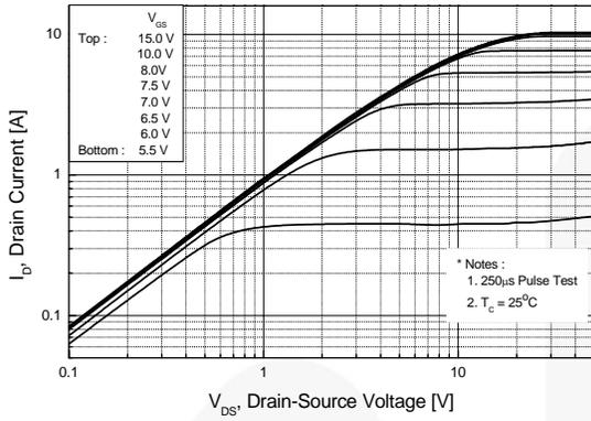
**Figure 2. Transfer Characteristics**
