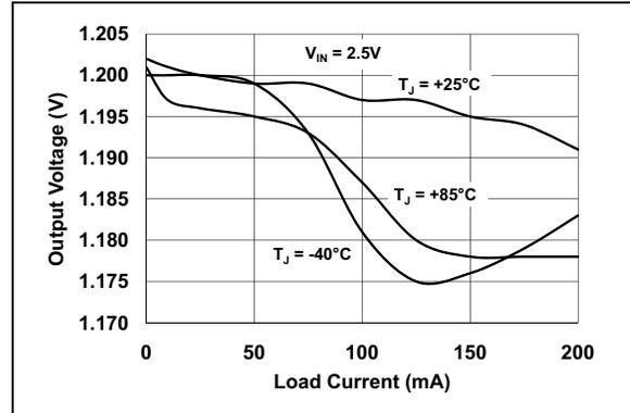
**FIGURE 2-4:** Output Voltage vs. Load Current ( $V_R = 1.2\text{V}$ ).
