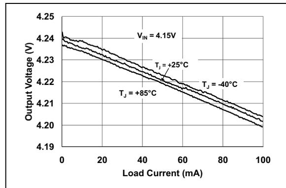
**FIGURE 2-6:** Output Voltage vs. Load Current ( $V_R = 4.2\text{V}$ ).
