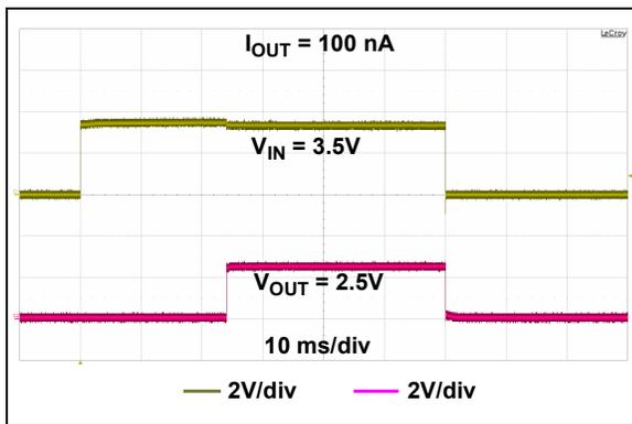
**FIGURE 2-20:** Start-up from  $V_{IN}$  ( $V_R = 2.5\text{V}$ ).
