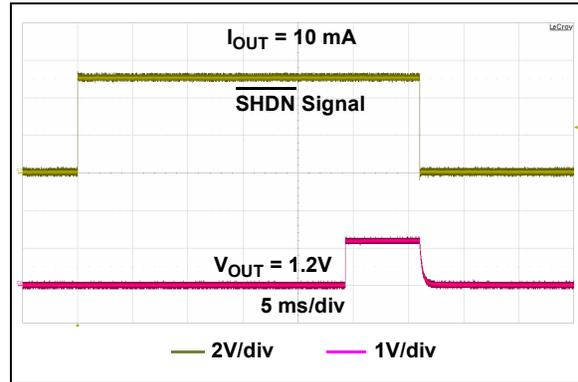
**FIGURE 2-22:** Start-up from SHDN ( $V_R = 1.2\text{V}$ ).
