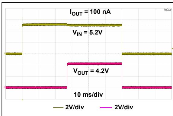
**FIGURE 2-21:** Start-up from  $V_{IN}$  ( $V_R = 4.2\text{V}$ ).
