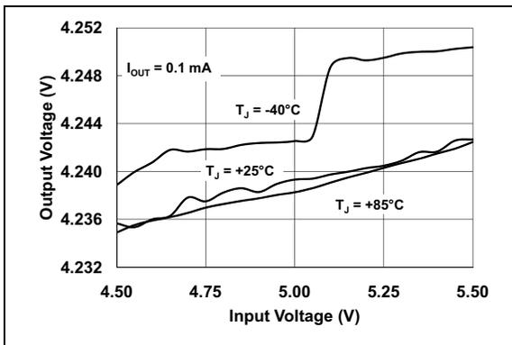
**FIGURE 2-3:** Output Voltage vs. Input Voltage ( $V_R = 4.2\text{V}$ ).
