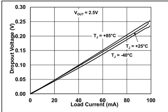
**FIGURE 2-7:** Dropout Voltage vs. Load Current ( $V_R = 2.5\text{V}$ ).
