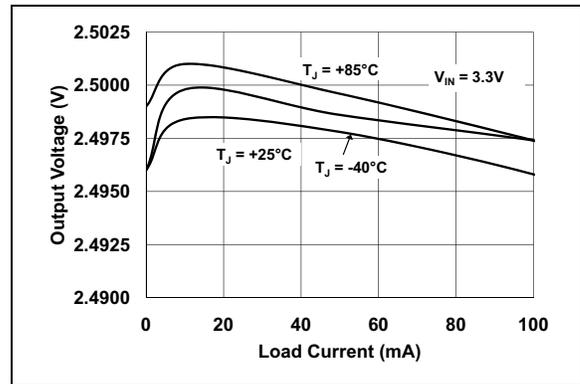
**FIGURE 2-5:** Output Voltage vs. Load Current ( $V_R = 2.5\text{V}$ ).
