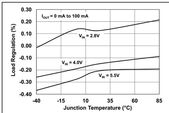
**FIGURE 2-26:** Load Regulation vs. Junction Temperature ( $V_R = 2.5\text{V}$ ).
