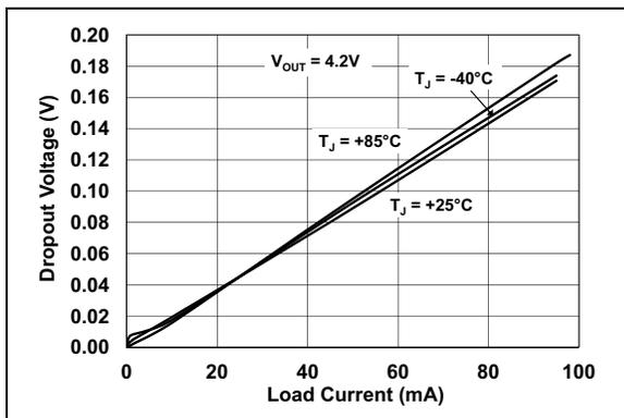
**FIGURE 2-8:** Dropout Voltage vs. Load Current ( $V_R = 4.2\text{V}$ ).
