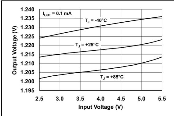
**FIGURE 2-1:** Output Voltage vs. Input Voltage ( $V_R = 1.2\text{V}$ ).
