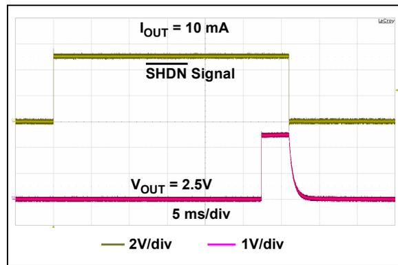
**FIGURE 2-23:** Start-up from SHDN ( $V_R = 2.5\text{V}$ ).
