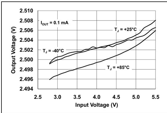
**FIGURE 2-2:** Output Voltage vs. Input Voltage ( $V_R = 2.5\text{V}$ ).
