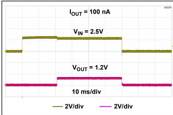
**FIGURE 2-19:** Start-up from  $V_{IN}$  ( $V_R = 1.2\text{V}$ ).
