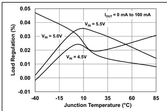
**FIGURE 2-27:** Load Regulation vs. Junction Temperature ( $V_R = 4.2\text{V}$ ).
