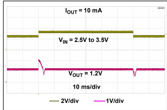
**FIGURE 2-16:** Dynamic Line Step ( $V_R = 1.2\text{V}$ ).
