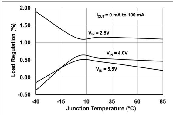
**FIGURE 2-25:** Load Regulation vs. Junction Temperature ( $V_R = 1.2\text{V}$ ).
