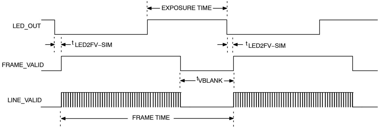
**Figure 13. Simultaneous Master Mode Synchronization Waveforms #1**
