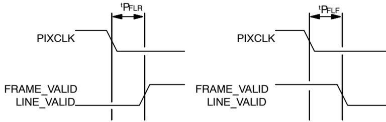
Figure 38. Propagation Delays for FRAME\_VALID and LINE\_VALID Signals
