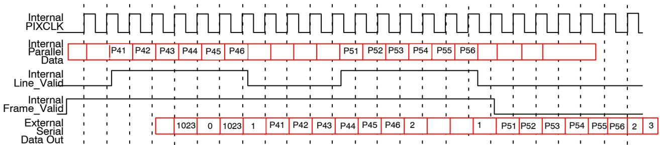
**Figure 35. Serial Output Format for a 6x2 Frame**
