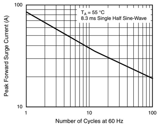
Figure 2. Maximum Non-Repetitive Peak Forward Surge Current
