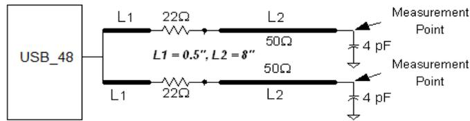
**Figure 8. Single-ended USB\_48 Clock Double Load Configuration**
