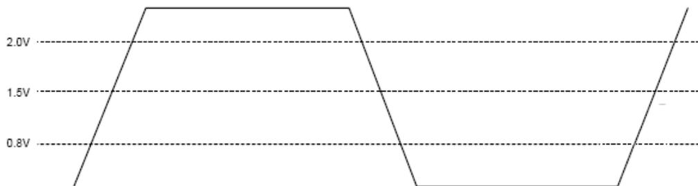
**Figure 10. Single-ended Output Signals (for AC Parameters Measurement)**
