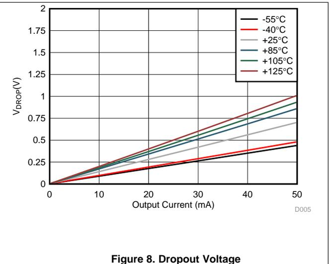
Figure 8. Dropout Voltage
