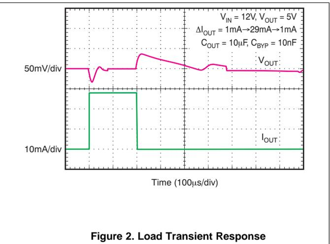
Figure 2. Load Transient Response
