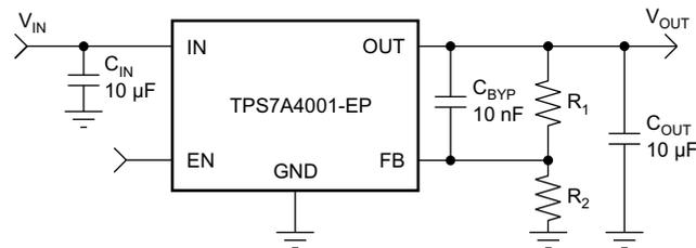
**Figure 13. Adjustable Operation for Maximum AC Performance**
