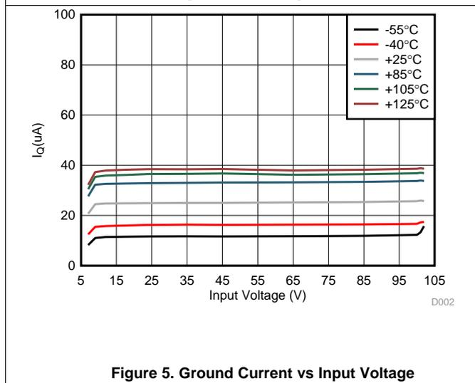
Figure 5. Ground Current vs Input Voltage
