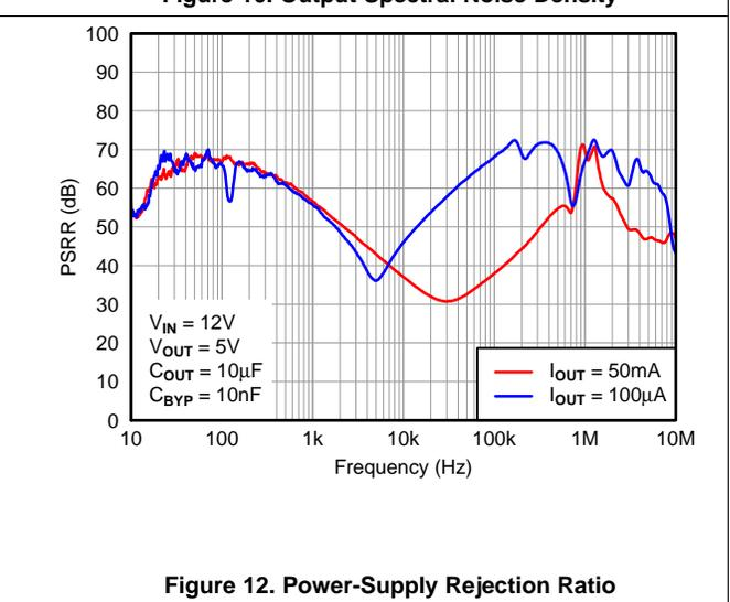
Figure 12. Power-Supply Rejection Ratio
