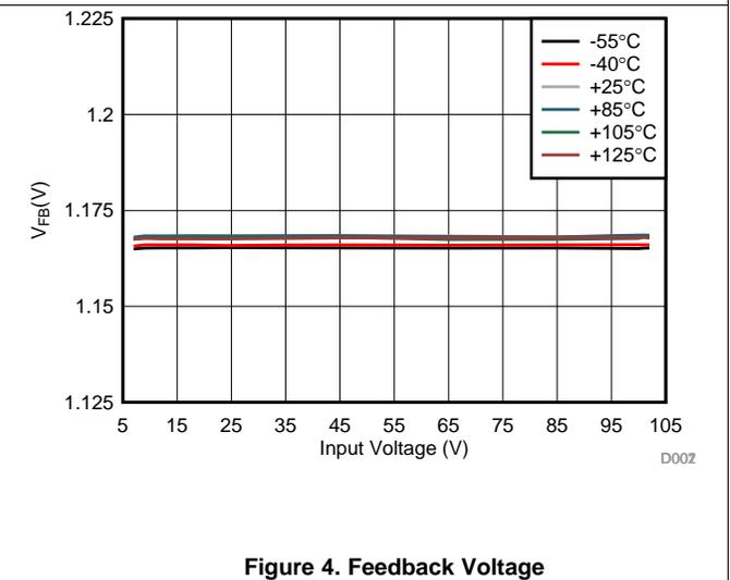
Figure 4. Feedback Voltage
