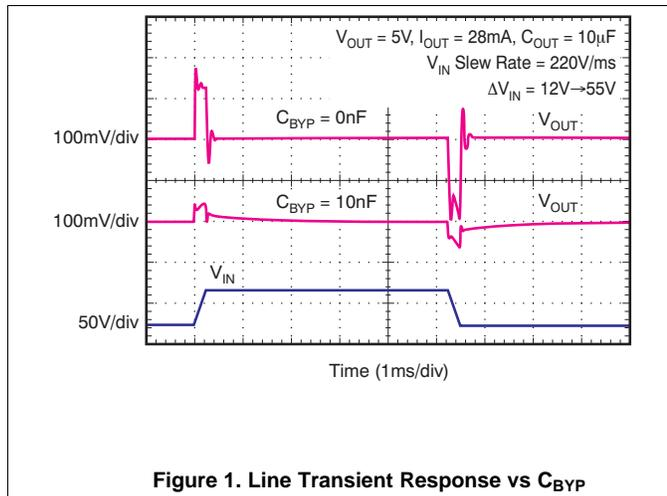
Figure 1. Line Transient Response vs  $C_{BYP}$
