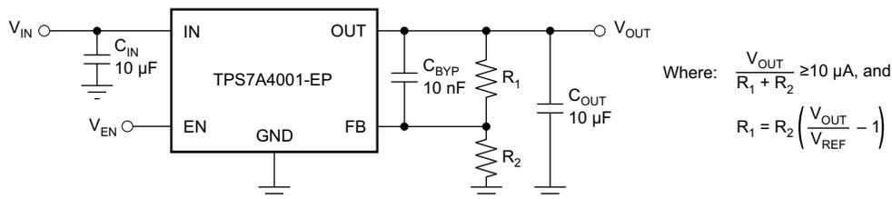
Figure 14. Example Circuit to Maximize Transient Performance
