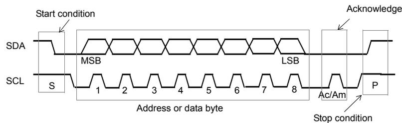
Information is packed in 8-bit packets (bytes) always followed by an acknowledge bit, Ac for VL53L3CX acknowledge and Am for master acknowledge (host bus master). The internal data is produced by sampling SDA at a rising edge of SCL. The external data must be stable during the high period of SCL. The exceptions to this are start (S) or stop (P) conditions when SDA falls or rises respectively, while SCL is high.
