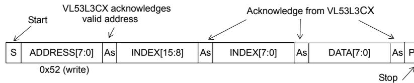
As data are received by the slave, they are written bit by bit to a serial/parallel register. After each data byte is received by the slave, an acknowledge is generated. The data are then stored in the internal register addressed by the current index.
