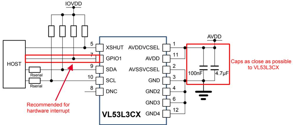
**Note:** Capacitors on the external supply AVDD should be placed as close as possible to the AVDDVCSEL and AVSSVCSEL module pins.
