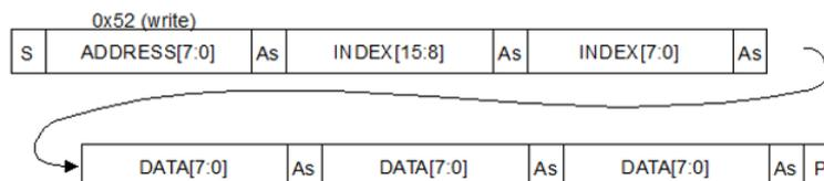
**Figure 14. VL53L3CX data format (sequential read)**
