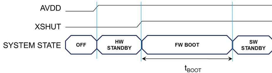
**Option 2:** The XSHUT pin is not controlled by the host, it is tied to AVDD through the pull-up resistor.
