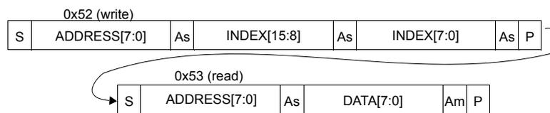
At the end of each byte, in both read and write message sequences, an acknowledge is issued by the receiving device (that is, the VL53L3CX device for a write and the host for a read).
