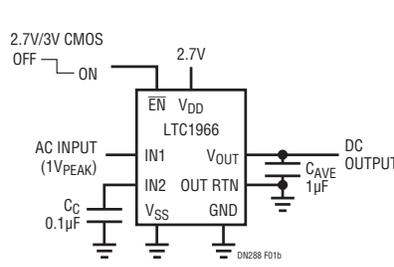
**Figure 1b. 2.7V Single Supply, Single Ended, AC-Coupled RMS-to-DC Converter with Shutdown**
