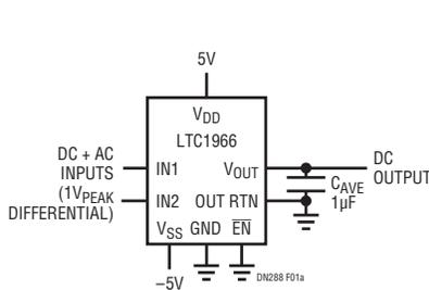
**Figure 1a.  $\pm 5V$  Supplies, Differential, DC-Coupled RMS-to-DC Converter**
