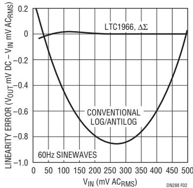
**Figure 2. Quantum Leap in Linearity Performance**
