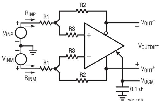
Figure 6. Input Impedance
