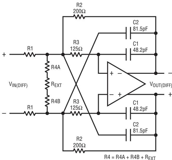
$$GAIN = \frac{V_{OUT(DIFF)}}{V_{IN(DIFF)}} = \frac{R2}{R1}$$
