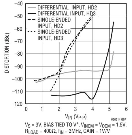
**Harmonic Distortion vs Input Common Mode Voltage ( $V_S = 3V$ )**
