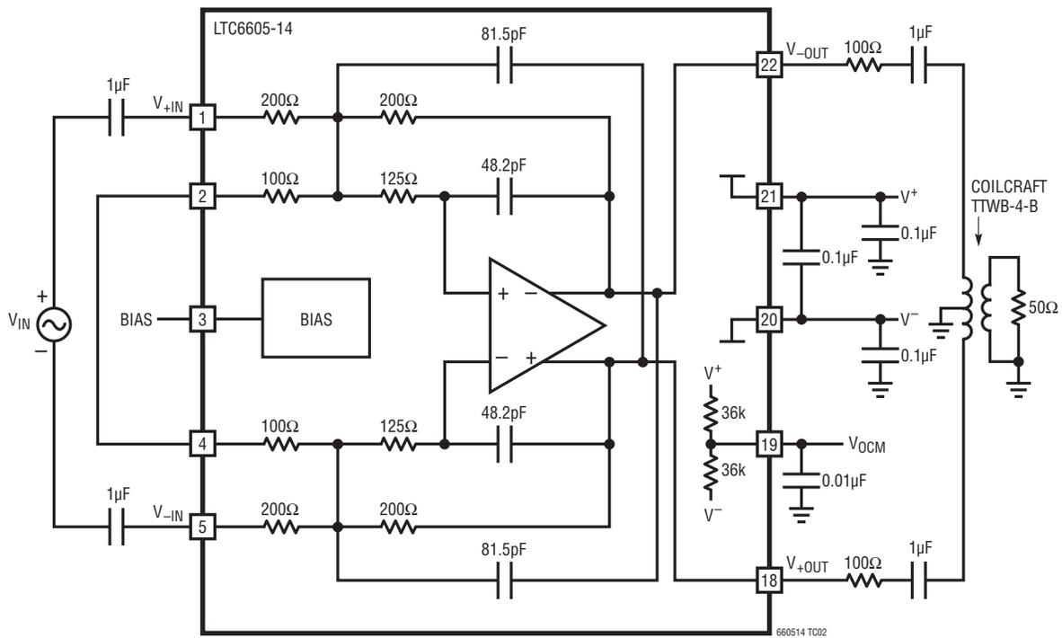
Figure 2. AC Test Circuit (Channel A Shown)
