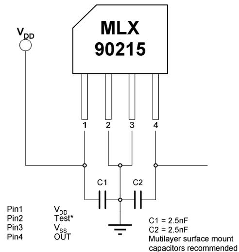
\*Readback diagnostic use only. Pin 2 is NOT for programming device. For best results, tie to GND.
