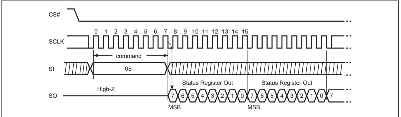
**Figure 12-2. Read Status Register (RDSR) Sequence (Command 05)**
