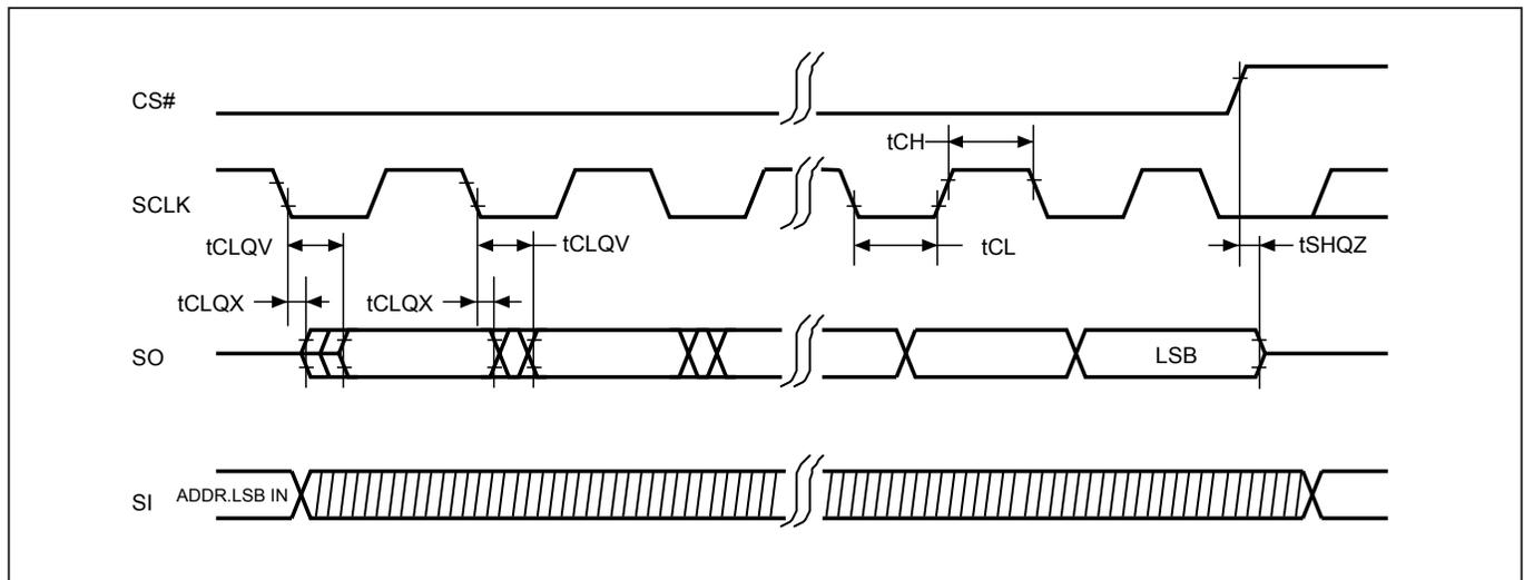
**Figure 8. WP# Disable Setup and Hold Timing during WRSR when SRWD=1**
