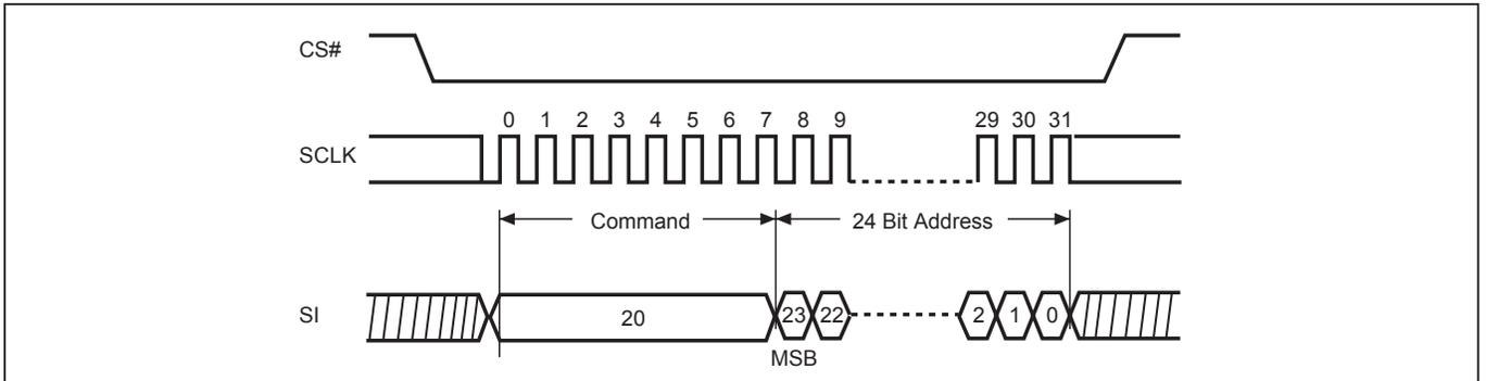
**Figure 17. Block Erase (BE) Sequence (Command D8 or 52)**
