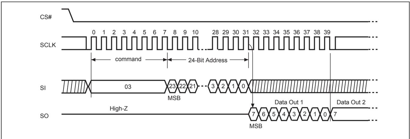
**Figure 15. Read at Higher Speed (FAST\_READ) Sequence (Command 0B)**
