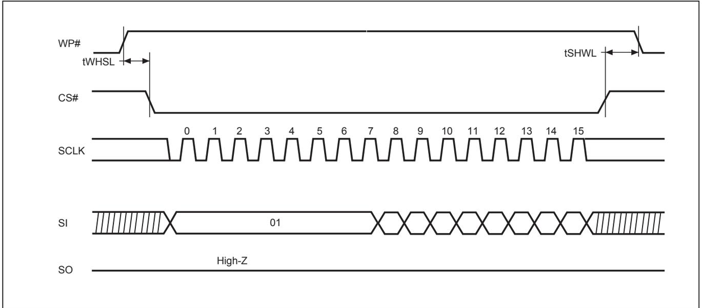
**Figure 9. Write Enable (WREN) Sequence (Command 06)**
