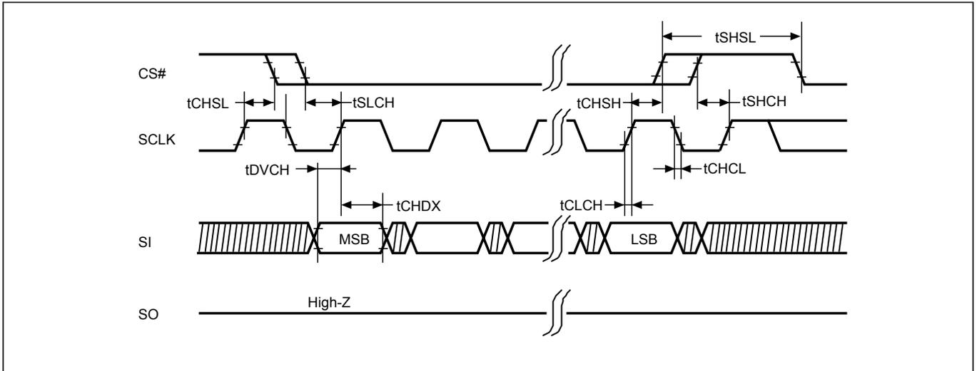
**Figure 7. Output Timing**
