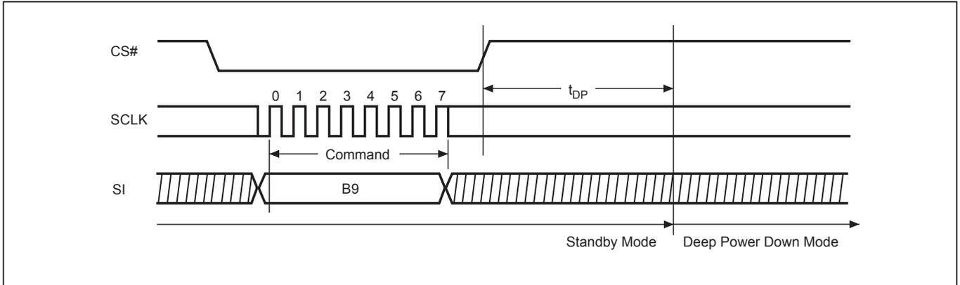
**Figure 21. Release from Deep Power Down (RDP) Sequence (Command AB)**
