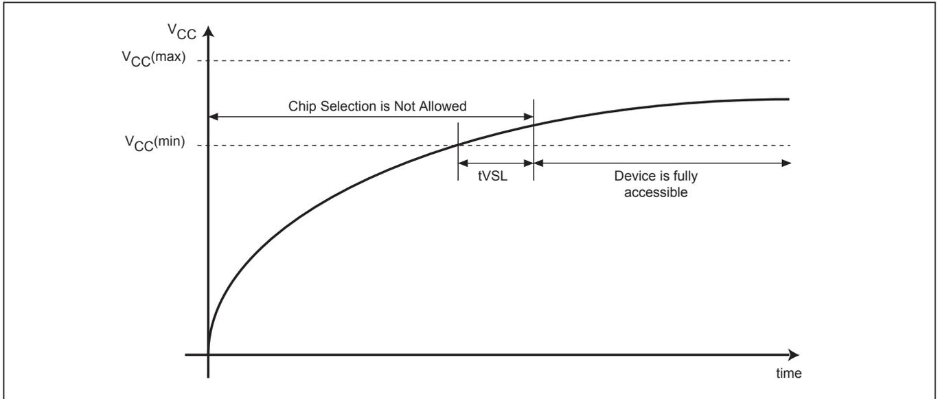
Note: VCC (max.) is 3.6V and VCC (min.) is 3.0V.
