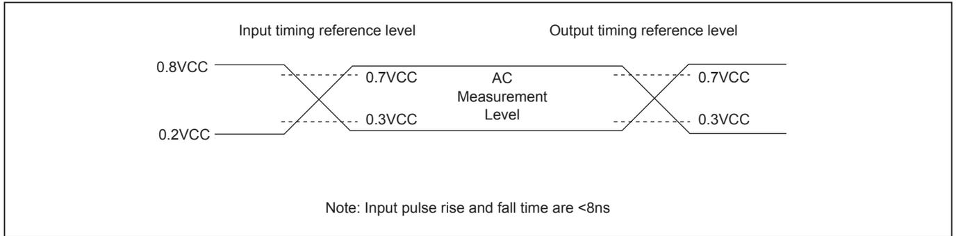
Notes: Rise time means 0.2VCC to 0.8VCC; Fall time means 0.8VCC to 0.2VCC.
