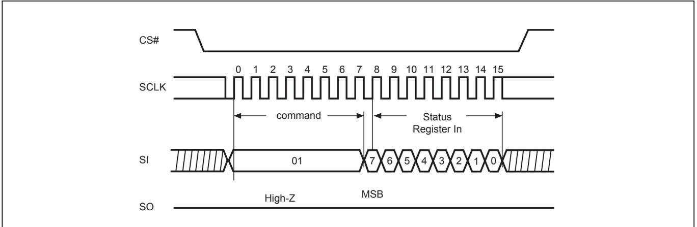
**Figure 14. Read Data Bytes (READ) Sequence (Command 03)**
