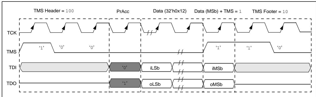
**FIGURE 6-8: XferFastData 2-WIRE (2-phase)**
