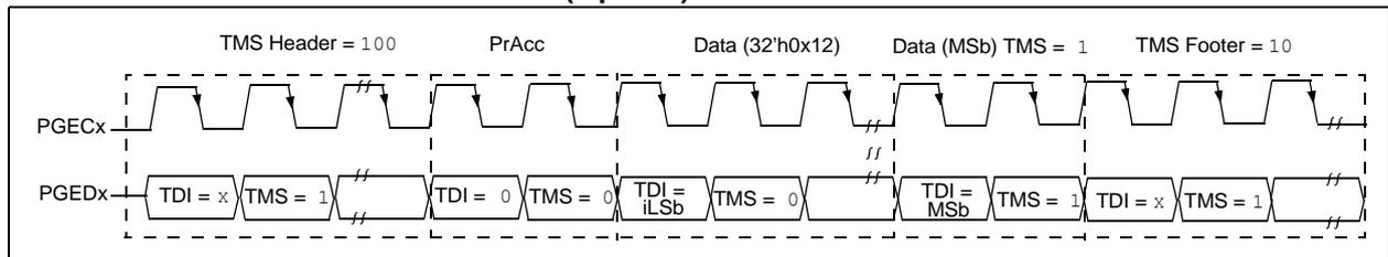
**FIGURE 6-9: XferFastData 2-WIRE (4-PHASE)**
