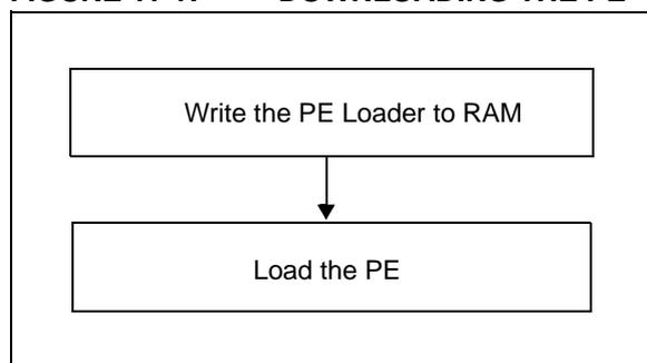
Loading the PE in the memory is a two step process:
