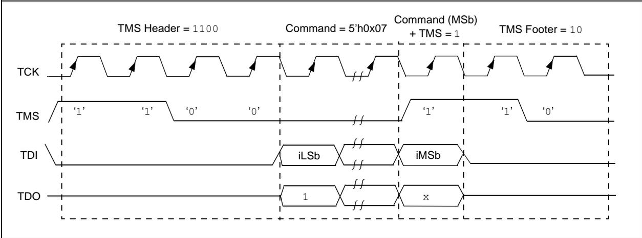
FIGURE 6-4: SendCommand 2-WIRE (4-PHASE)
