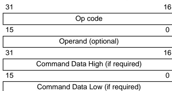
The command in the op code field must match one of the commands in the command set that is listed in Table 17-2. Any command received that does not match a command the list returns a NACK response, as shown in Table 17-3.
