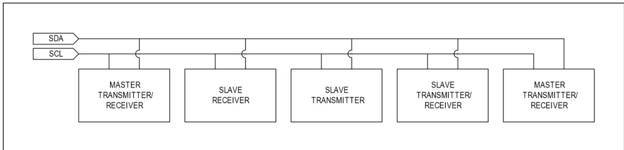
Figure 2. I<sup>2</sup>C system configuration.
