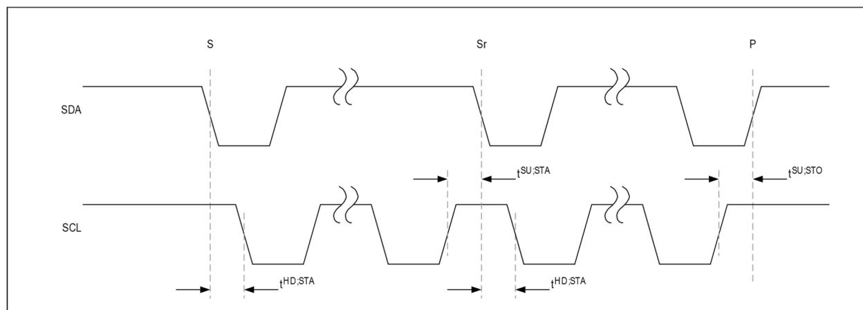
Figure 3. I<sup>2</sup>C START and STOP conditions.
