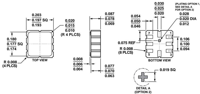
Figure 6. 8-Terminal Ceramic Leadless Chip Carrier [LCC] (E-8-1)
