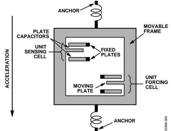
Figure 5. Simplified View of Sensor Under Acceleration
