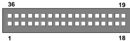
Figure 1. Pin Configuration for the 36-Way Connector, J1.
