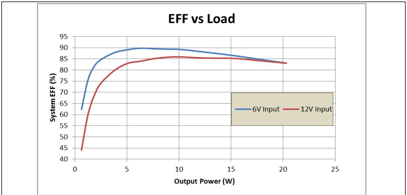
**Figure 2** System efficiency with VO= 2.5V, FSW=800kHz, Tj=45°C
