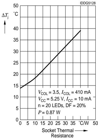
Max. Package Power Dissipation, ISD201X
