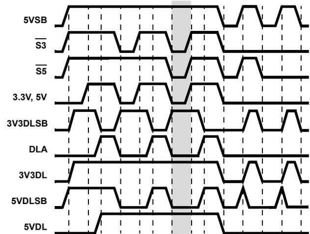
**FIGURE 5. 5V<sub>DUAL</sub> AND 3.3VDUAL/3.3V<sub>SB</sub> TIMING DIAGRAM; EN5 = 5V/OPEN**
