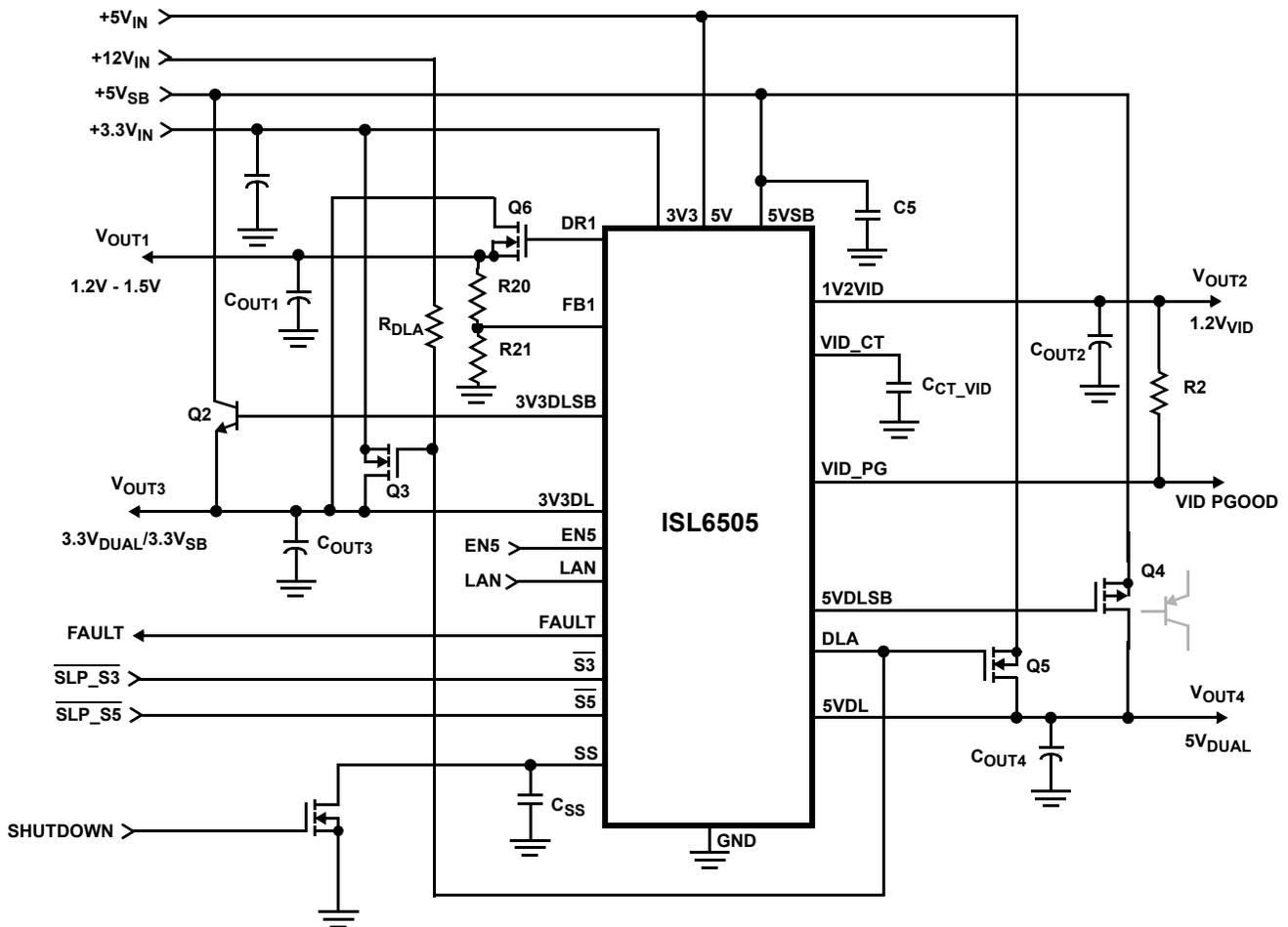
V<sub>OUT1</sub> = 1.2V to 1.5V: Q6 = FDD6530A, C<sub>OUT1</sub> = 1000μF
