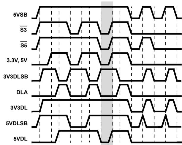
**FIGURE 4. 5V<sub>DUAL</sub> AND 3.3VDUAL/3.3V<sub>SB</sub> TIMING DIAGRAM; EN5 = GND**
