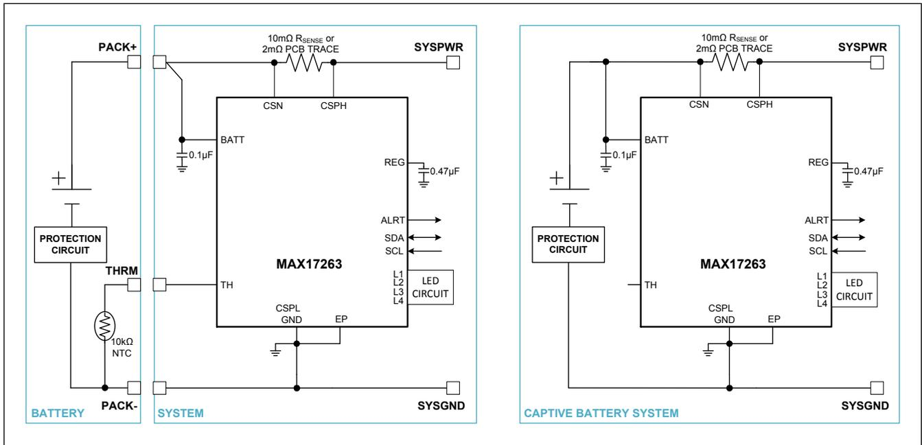
Figure 8. High-Side Current Measurement Typical Applications Circuit
