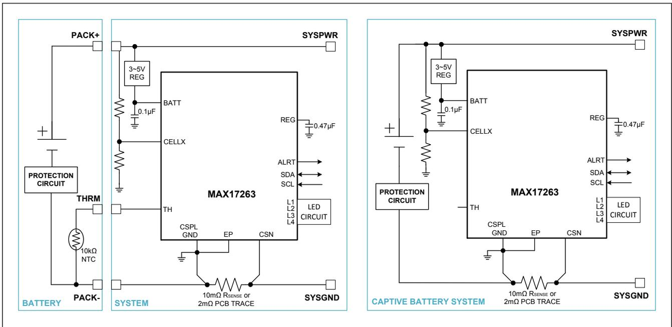
Figure 6. Multi-Cell Low-Side Current Measurement Typical Applications Circuit
