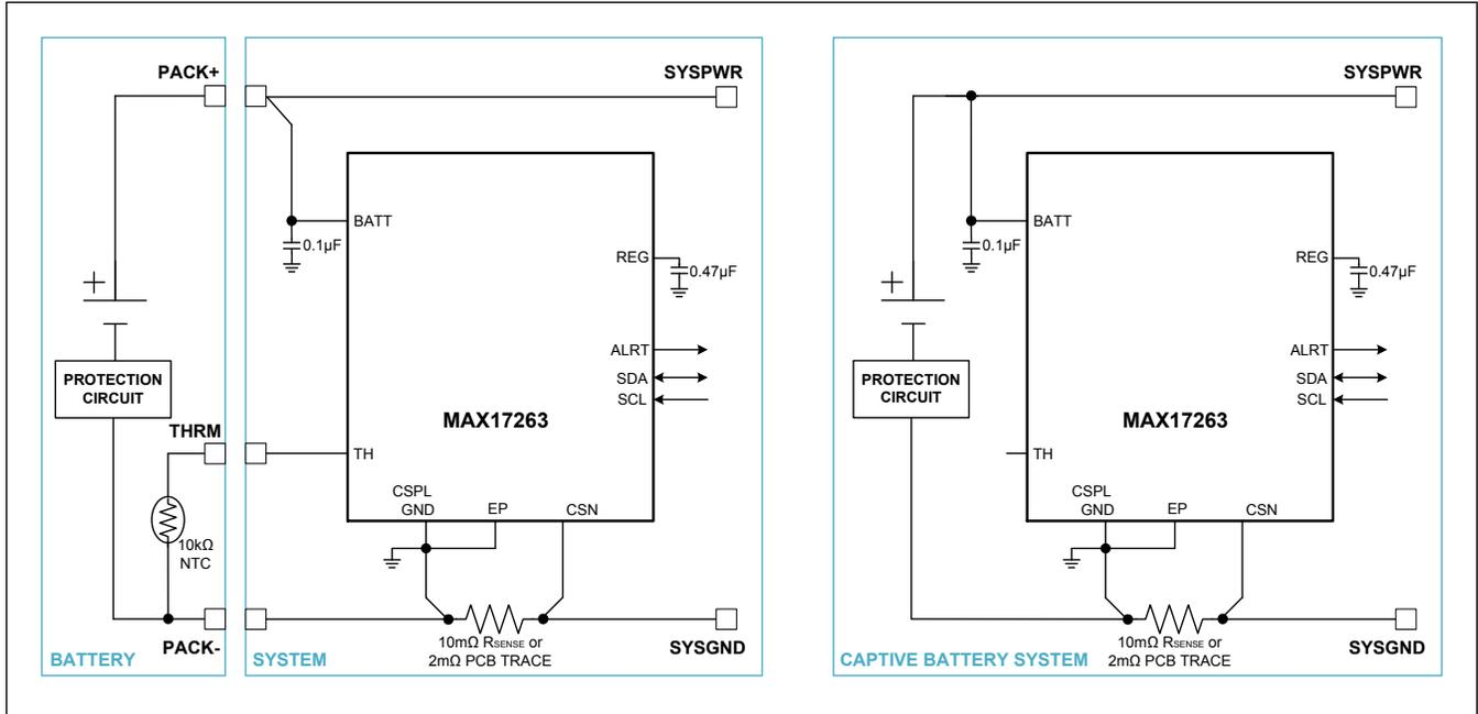
Figure 7. Single-Cell Low-Side Current Measurement Typical Applications Circuit
