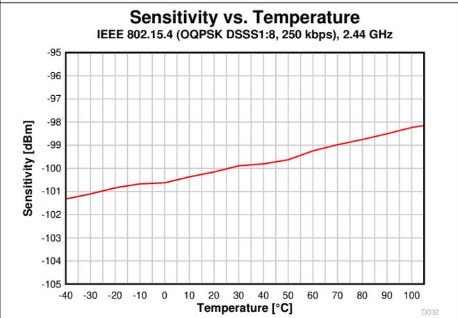
Figure 7-17. Sensitivity vs. Temperature (250 kbps, 2.44 GHz)
