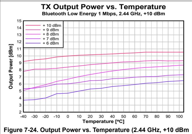
Figure 7-24. Output Power vs. Temperature (2.44 GHz, +10 dBm PA)
