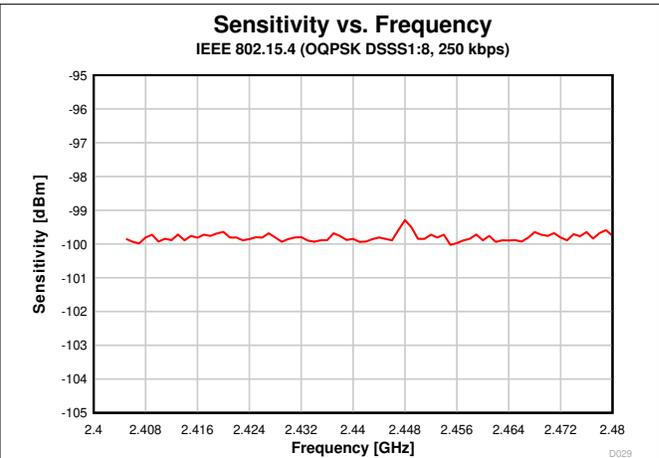
Figure 7-15. Sensitivity vs. Frequency (250 kbps, 2.44 GHz)
